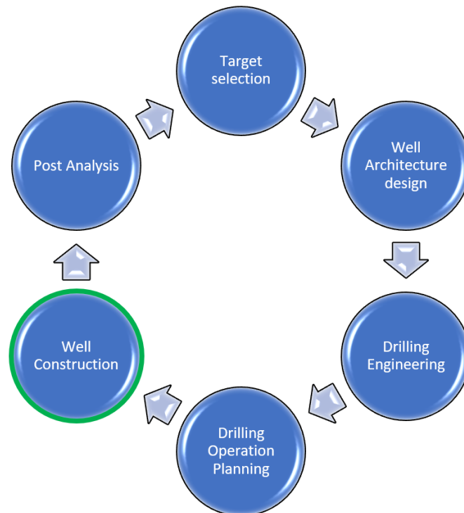
Fig. 11: Schematic representation of the well construction life cycle. Each of these tasks have their own requirements for modelling of the drilling process. In the context of this thesis, we focus on the requirements for modelling during the construction part of the cycle, i.e. for real-time applications.
