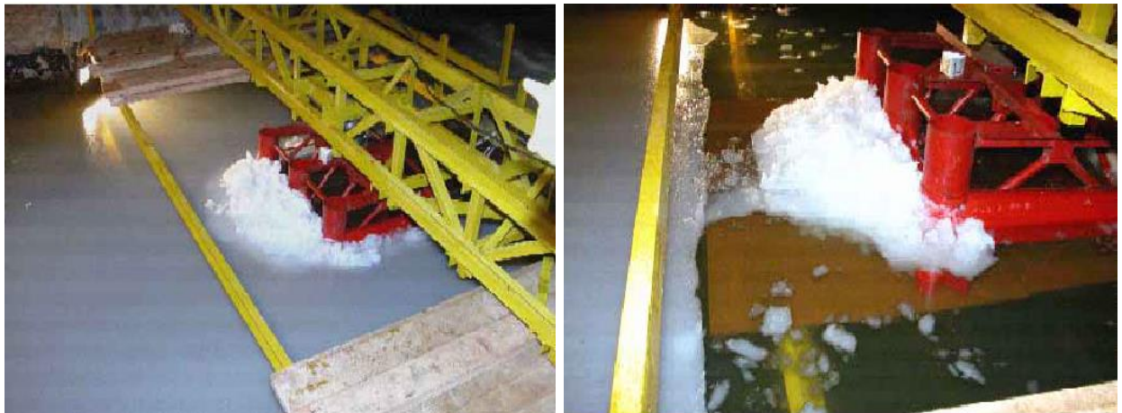
Fig. 2.5 Forming ice rubble accumulations in front of IRP-1 model [13]
