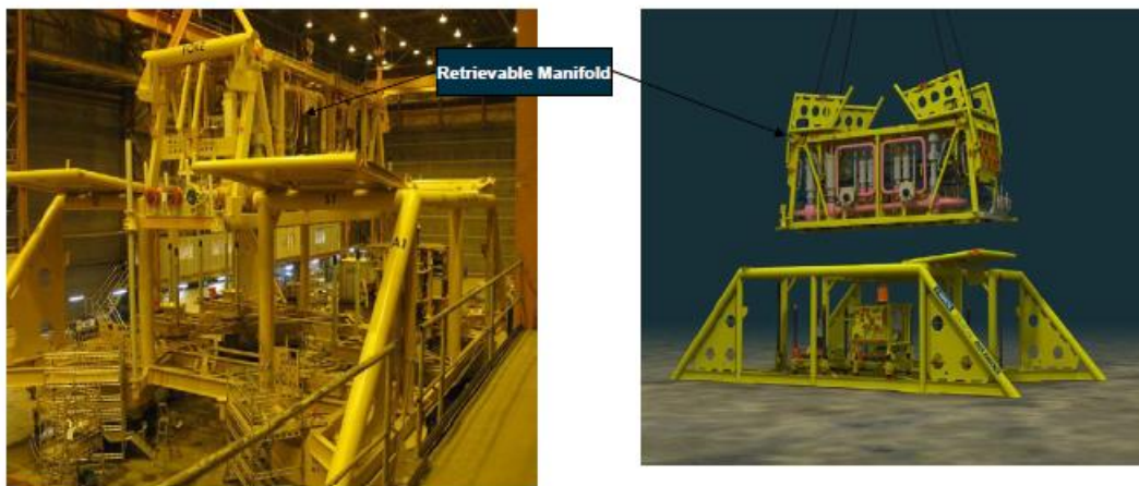
Figure 4.18. Integrated production template [59]
