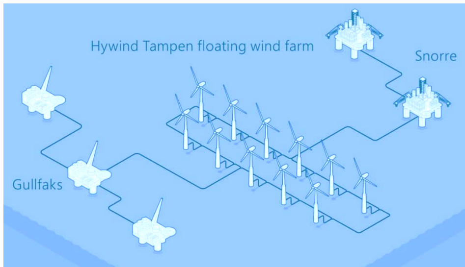
Illustration 6: An illustration of Hywind Tampen which shows how the floating turbines will give power to the oil fields Gullfaks and Snorre. Source: Oljedirektoratet, 2019.
