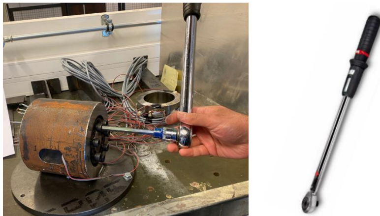
Figure 4.8: Application of torque using USAG torque wrench
