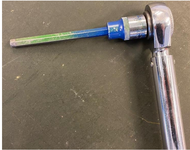
Figure 6.10: Fixture used with torque wrench
