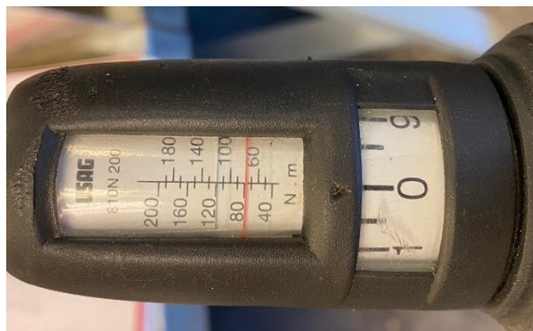
Figure 4.7: Dial of USAG torque wrench indicating range from 40 to 200 Nm
