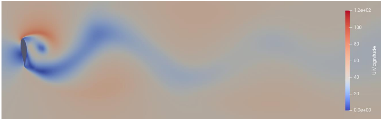
Figure 74: Flow over the turbine blade, Course Mesh, cross section at 60m
