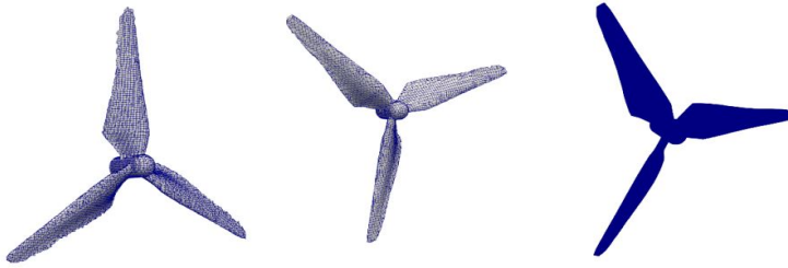
Figure 5.6: Analysis of grid study (From left: Coarse,Mild and Very fine).
