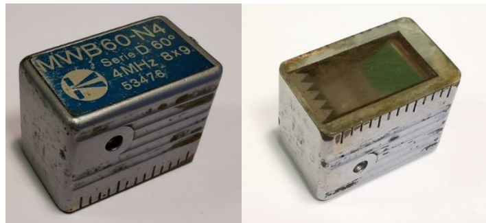
Figure 3-1 MWB60 - N4 ultrasonic probe The right picture is a top view and the left one is a bottom view of the probe
