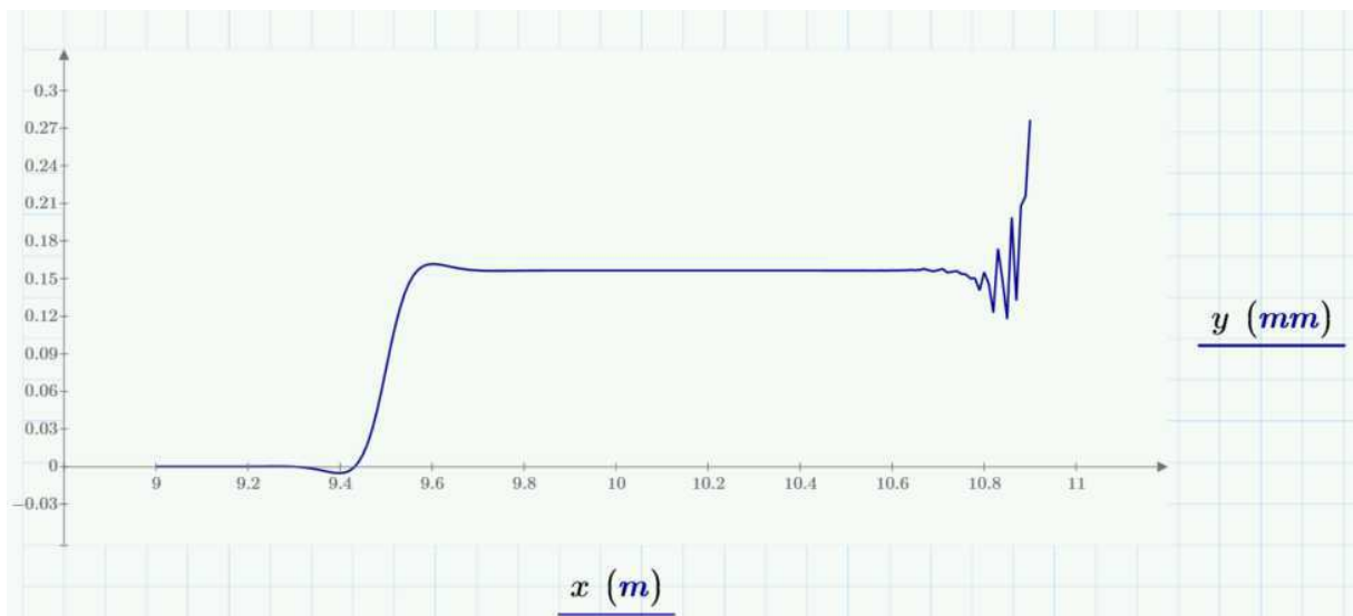
Fig. 28 – Radial deflection of a thin-walled cylindrical shell, calculated in Section 5.4.
