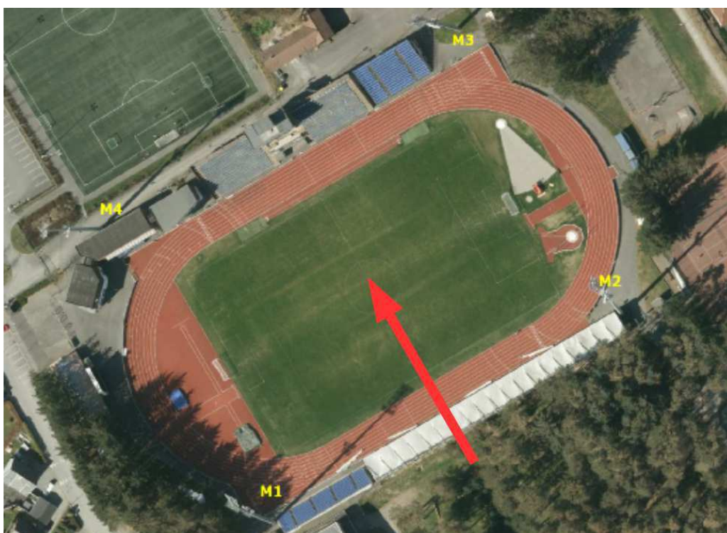
Fig. 6 – Principal dominant wind direction, SSE, at site, with the four masts denoted M1, M2, M3 and M4.
