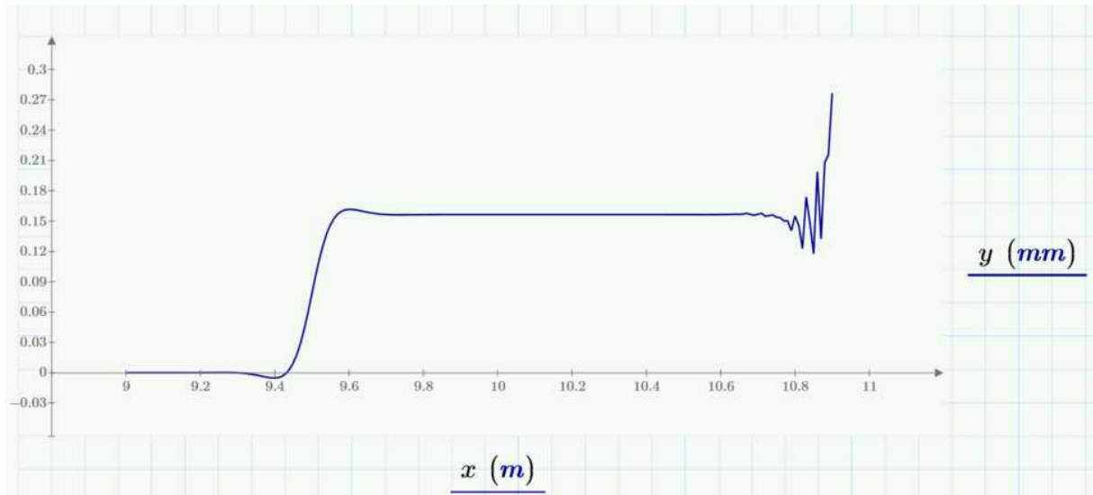
Fig. 11 – Plotted radial deflection, 9000 mm from the free end to the end of the segment (11,100 mm).
