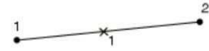
Fig. 33 – A 2-node linear beam element with node numbers and one integration point (Dassault Systemes, 2019).
