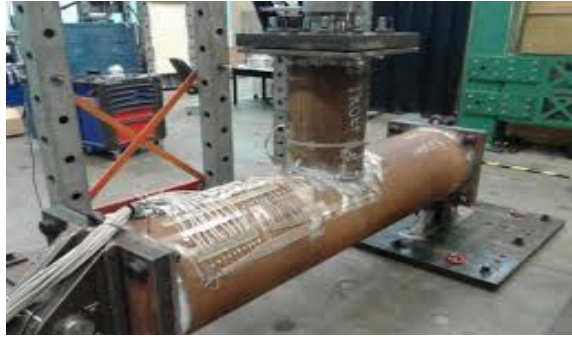
Figure 2.12: Tubular T-joint test. [8]
