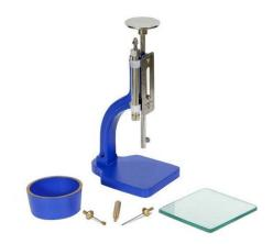
FIGURE 3.5: Vicat test apparatus and its attachments
