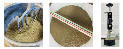
FIGURE 4.4: Blending dry material and immediately after tests
