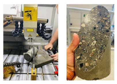
FIGURE 4.3: Cutting process and the cut specimen
