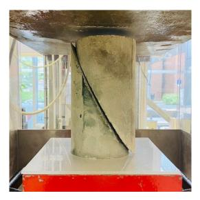
FIGURE 4.6: A collapsed slant shear specimen
