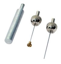
FIGURE 3.6: Vicat test needles
