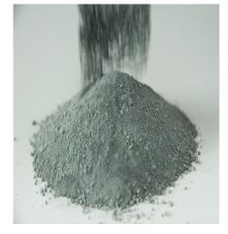
FIGURE 3.1: The micro silica in use.
