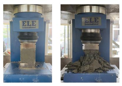
FIGURE 4.5: A cubic specimen collapsed under applied load.
