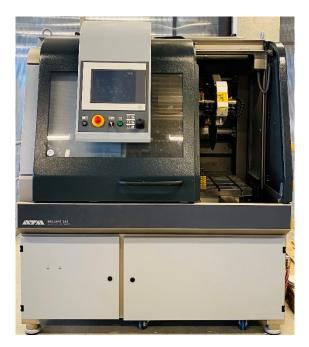
FIGURE 4.2: Cutting machine ATM Brilliant 285
