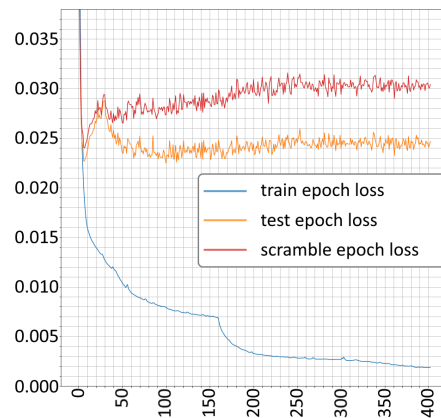
Figure 5.29: Graphs showing the MSE test losses during training when the segmentation model uses a fully connected layer connecting the down-stack and up-stack. See figure 5.28 for the segmentation model (not including the fully connected layer).
