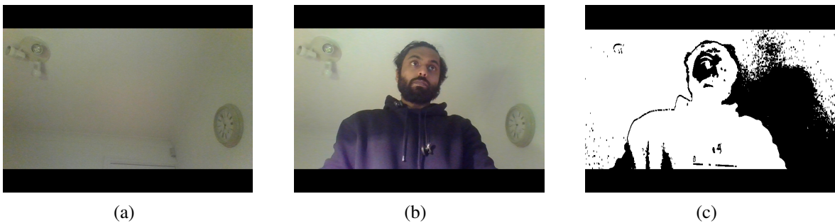
FIGURE 3.1. Absolute difference between the image (a) and image (b) shown in (c)
