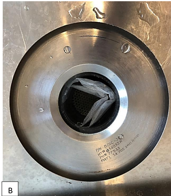
Figure 15: A) The plastic bag was filled with 6 grams of tuna fish solution, sealed with the Dyno packaging machine and rolled flat. B) The plastic bags inside the pressure chamber of the PATS for processing at pressure of 600MPa combined with 55 °C and 65 °C for 2 minutes, three parallels at a time.
