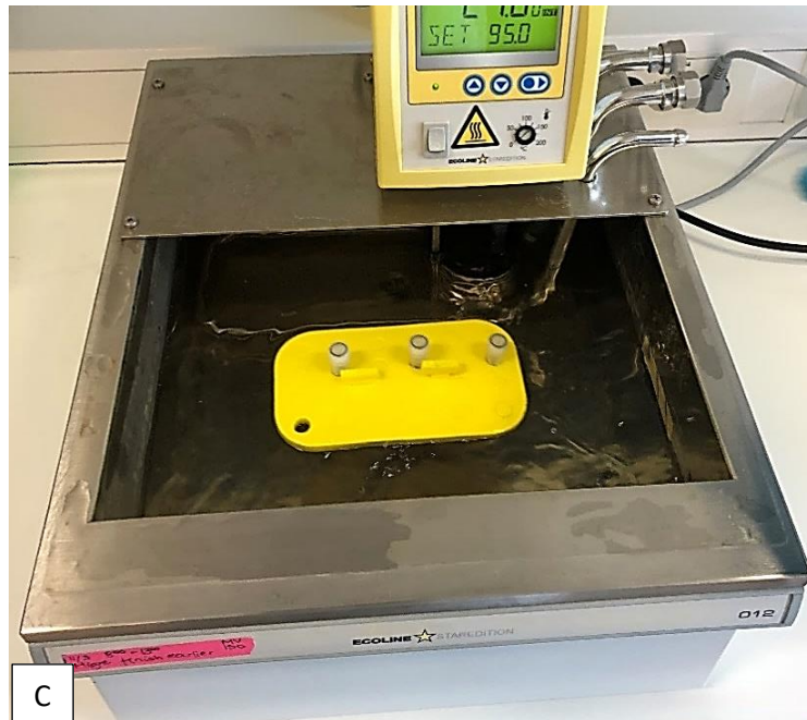
Figure 10: Equipment used in the water bath experiments. a) Screw cap tube ( Nunc tube), b) Temperature detector, and c) A floating element holds the nunc tubes in water bath for heat treatment.
