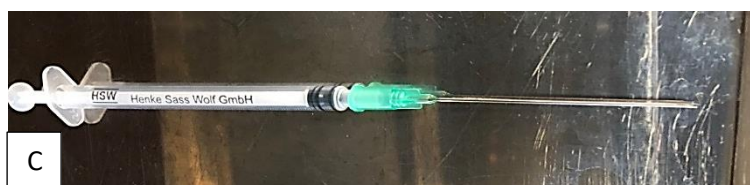
Figure 12: Equipment used in the water bath experiments. a) A metal rack holds the glass tubes in water bath for heat treatment, b) A glass tube with a rubber stopper and c) Sterile syringe that used to inoculate the samples into the glass tubes.
