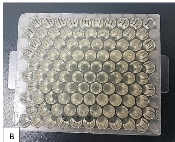
Figure 11: Equipment used for the growth experiment. a) Bioscreen C used to read the growth process and b) Honeycomb microtiter plate of 10 × 10 wells that is used in the Bioscreen C.
