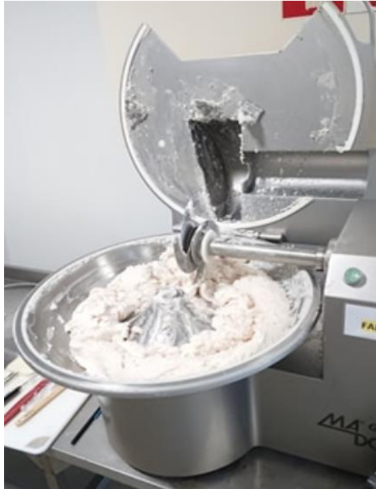
Figure 3.7. All ingredients of the minced fish were blended in an industrial cutter during pilot production.
