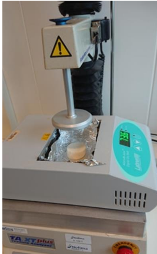
Figure 3.9. Texture profile analysis of minced fish product by using a compression plate and a heat block.
