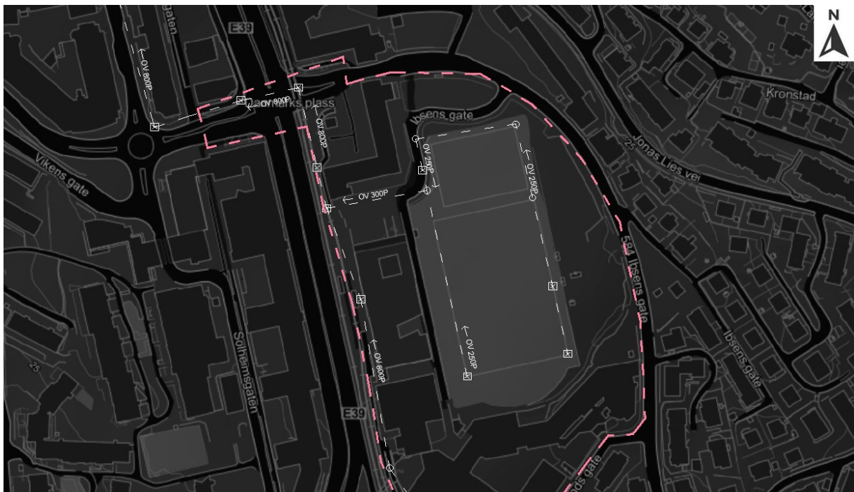
Figure 37 - New stormwater pipes Created by Eirik Instanes in Autocad
