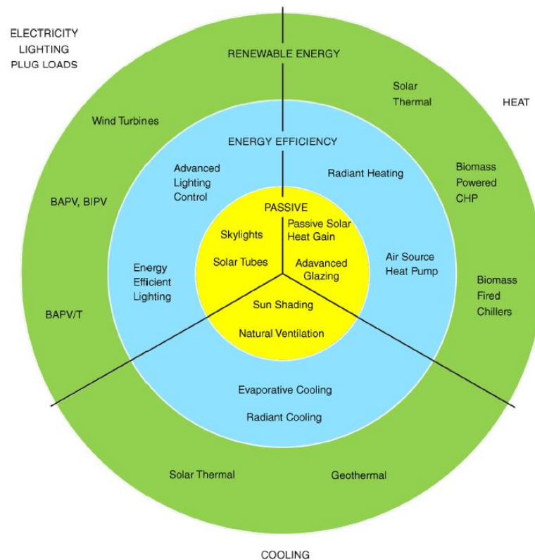
Fig. 3.4: Net ZEB design: Out progression and measure examples (Grade et al.,2017 p.17)
