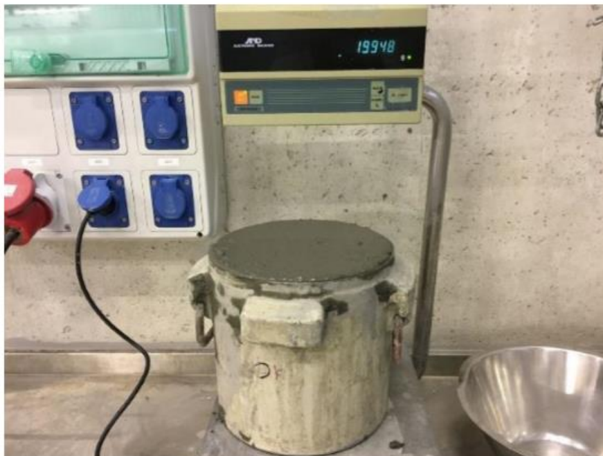
Figure 17 Air content and Density measurement
