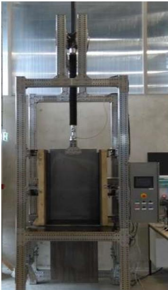
Figure 12 Slip form rig
