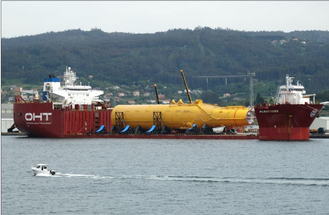
Figure 2.9 Transportation of a spar substructure used for Hywind Scotland [28].
