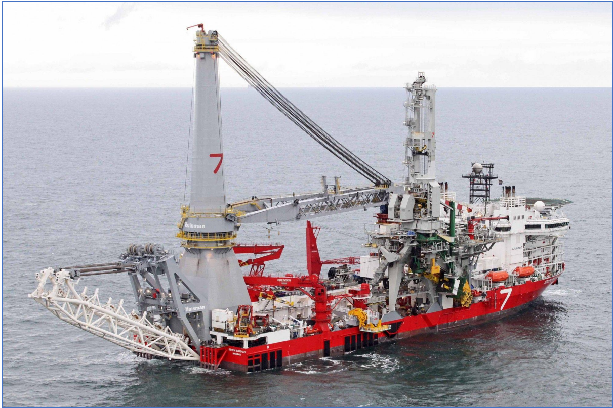
Figure 6-1 Seven Borealis pipe-layer and heavy lift vessel for Subsea 7
