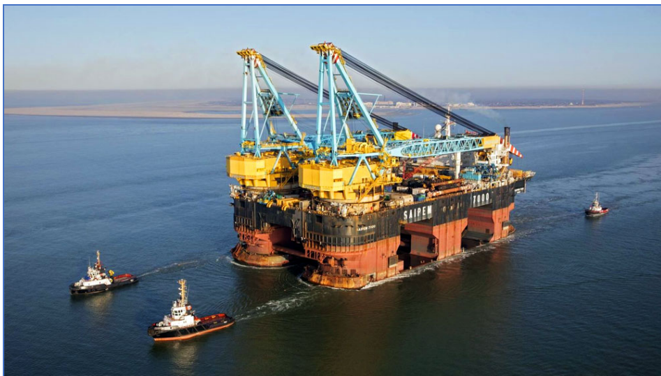
Figure 6-8 Saipem 7000 capable of lifting 14000tonnes
