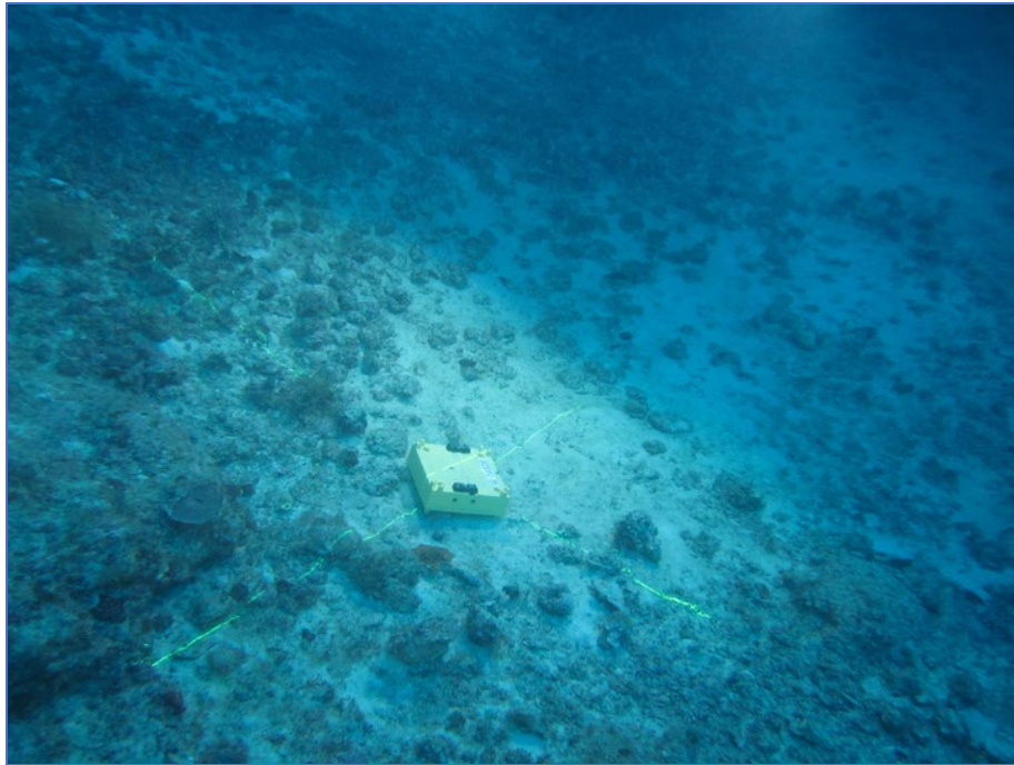
Figure 4-4 A manta nodes placed on seabed (Seabed Geosolutions)
