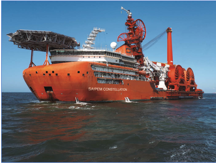
Figure 6-9 Saipem Constellation pipelay vessel
