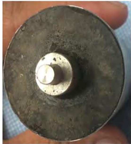
Figure 45: Typical shale radial strain behaviour observed during tests, with fast primary creep followed by slower secondary creep; (right) the ultimate result of creep, with an annulus around the central casing rod insert that has become completely blocked off with shale material
