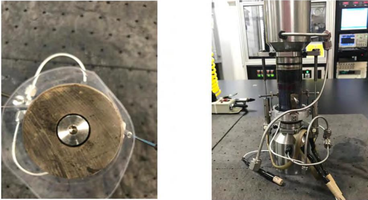
Figure 43: Left: top view of cylindrical shale sample with concentric casing insert before testing; (right) mounted shale sample in the test cell with cantilever bridge for strain measurement and upstream and downstream reservoirs with their pressure lines.
