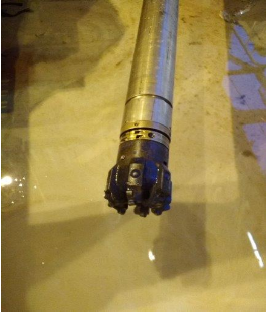
Figure 24: Milling bit 3.5" used to mill the scale
