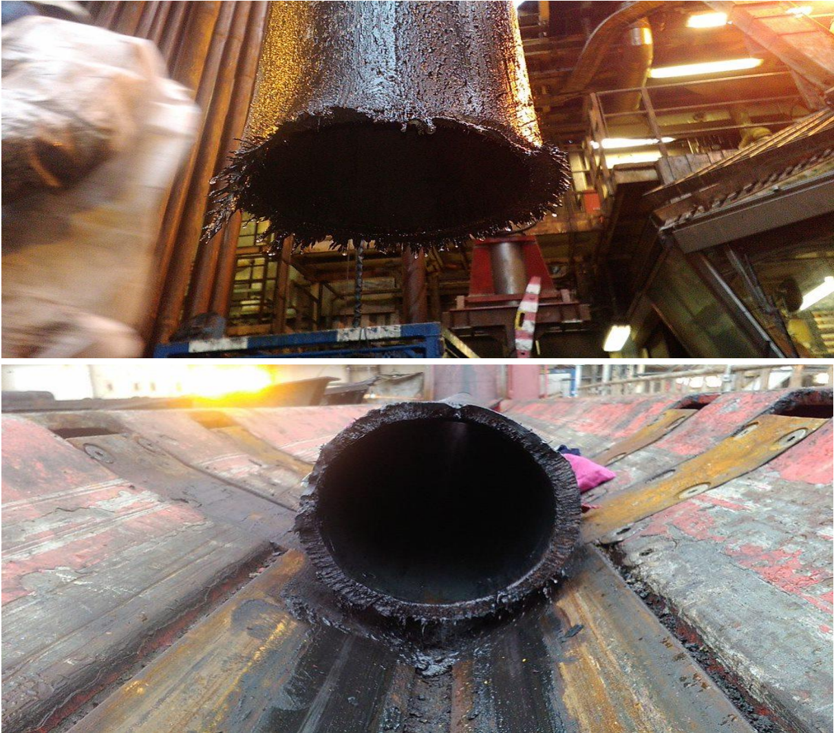
Figure 27: The pictures show a tubing cut for well A-32D at 4405 meters. There are no pictures for well A-27 lower cutting since the phase 2 was suspended due to corona virus.
