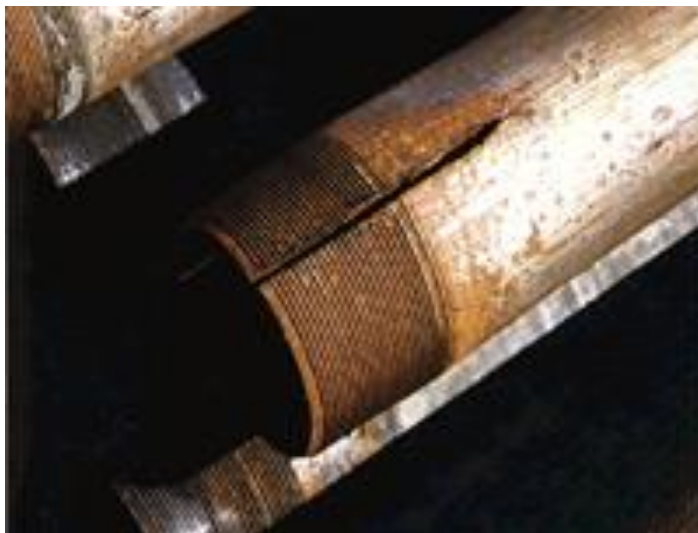
Figure 16: Split shot result on tubing (Halliburton)
