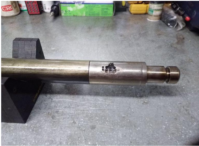
Figure 15: Plasma cutter tool used to make a hole in TBG (Repsol)
