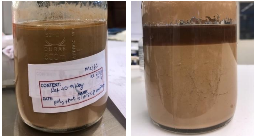
Figure 5.10: Free fluid accumulated at surface after ~1 day
