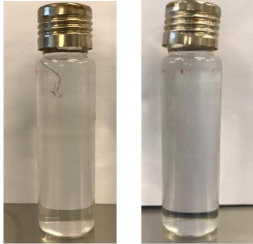
Figure 4.8: Silica solution dispersed in water, immediately (left) and after 24 hours (right)
