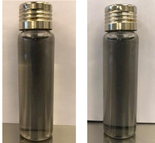
Figure 4.7: MWCNT-COOH solution dispersed in water, immediately (left) and after 24 hours (right)
