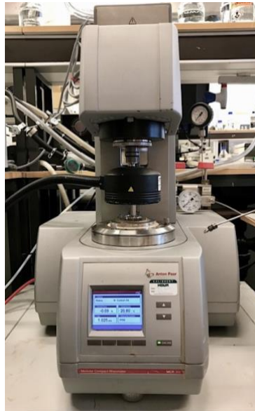
Figure 4.12: Anton Paar MCR 302 rheometer with parallel plate setup
