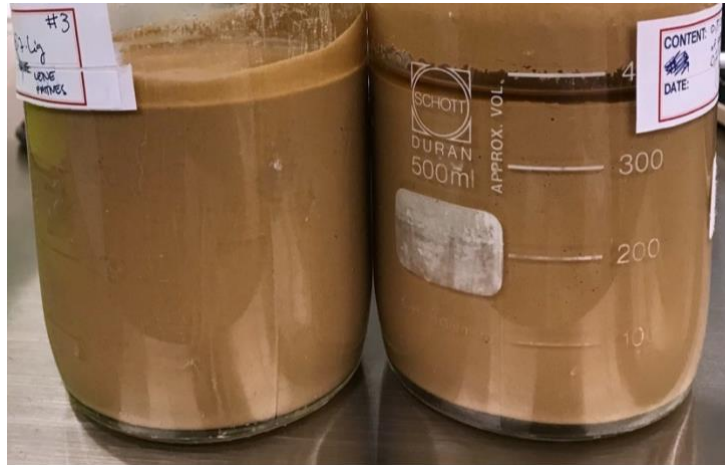
Figure 5.9: Free fluid accumulating at the surface after ~1 hour
