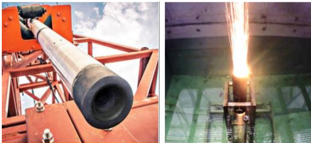
Figure 4-5: Left: PlasmaBit BHA on a test rig. Right: PlasmaBit milling during an inhouse laboratory test [27]
