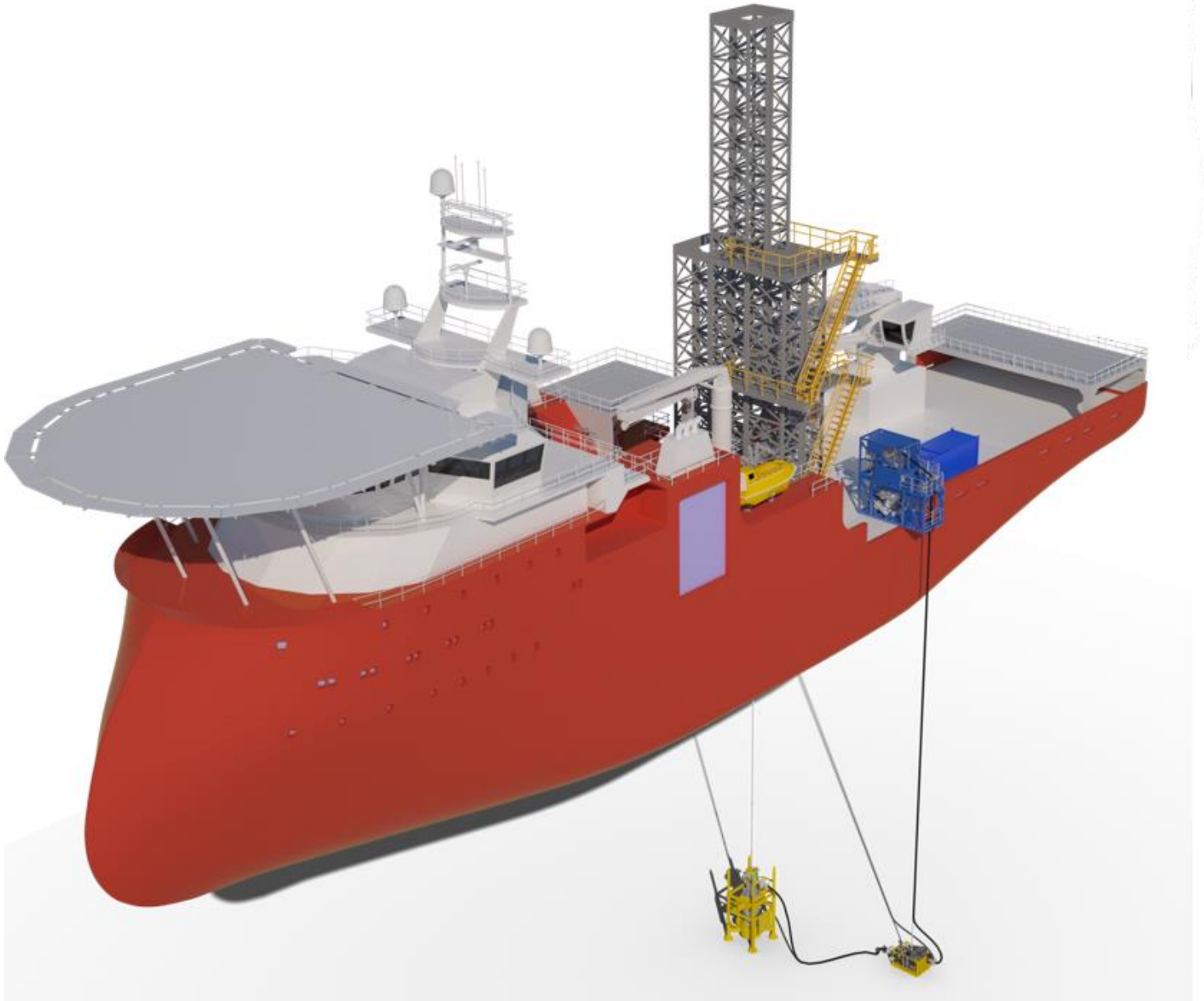
Figure 5-21: Volume control system installed on an LWI vessel. [67]
