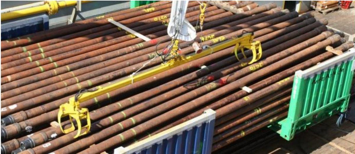
Figure 5-30: Lifting beam grabbing pipes from pipe storage rack. [64]
