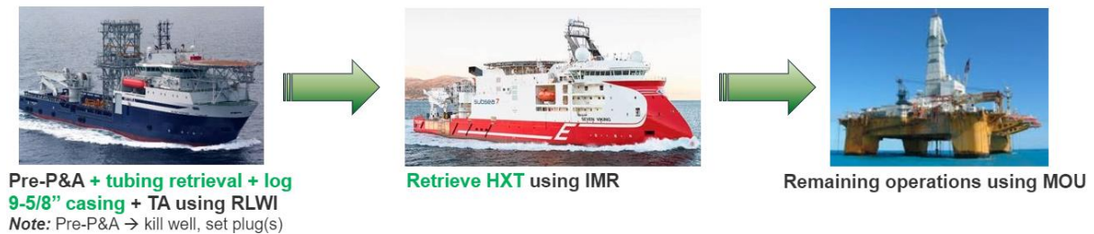
Figure 4-3: Proposed new unit selection for P&A operations on subsea wells with HXT [21]
