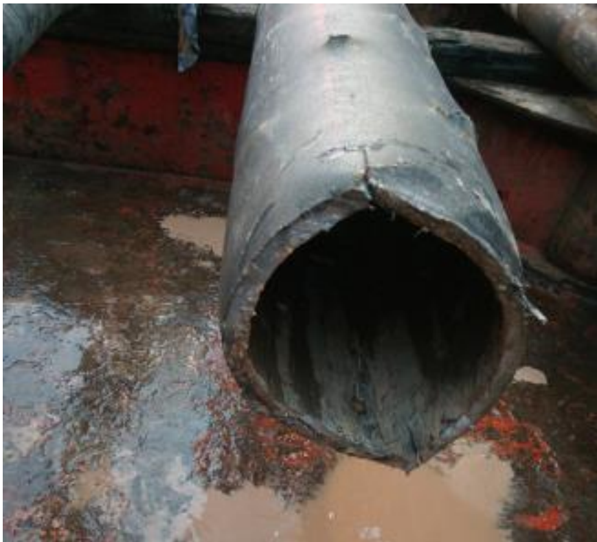
Figure 5-17: Tubing cut with NorOilTools surface cutting tool. [60]
