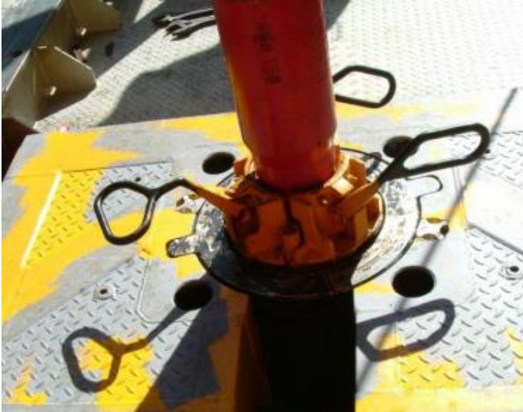
Figure 5-26: False rotary table with insert slips with colour coating as specified according to OLF 070 [64]
