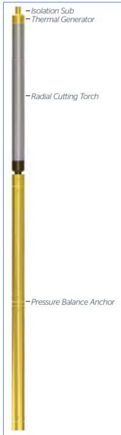
Figure 5-16: Example of a RCT BHA. [57]
