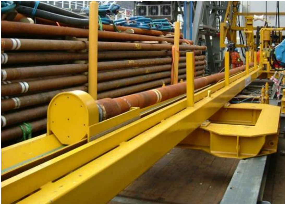
Figure 5-28: Travelling trolley with drill pipe in the gutter. The pipe storage rack in the background will be placed on the mezzanine as shown in figure 5-3. [64]
