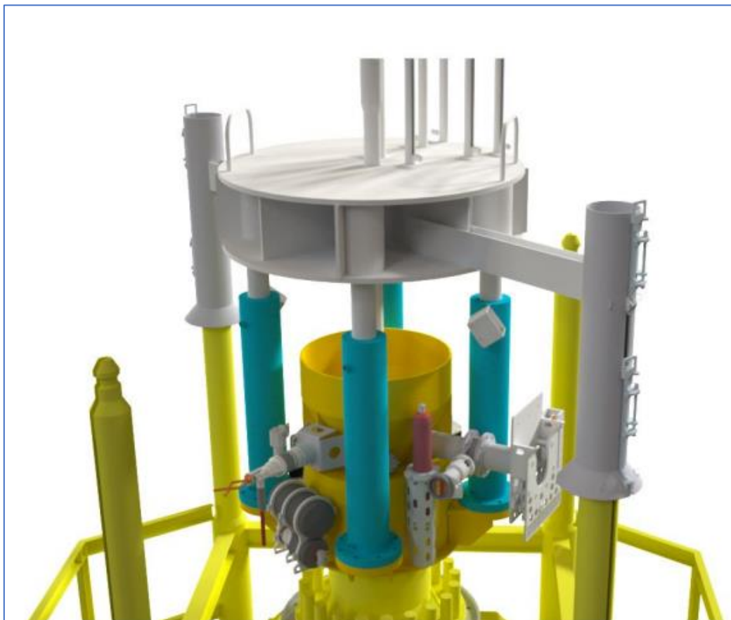
Figure 5-25: Subsea tubing hanger release jack installed on top of the WHIM. [63]
