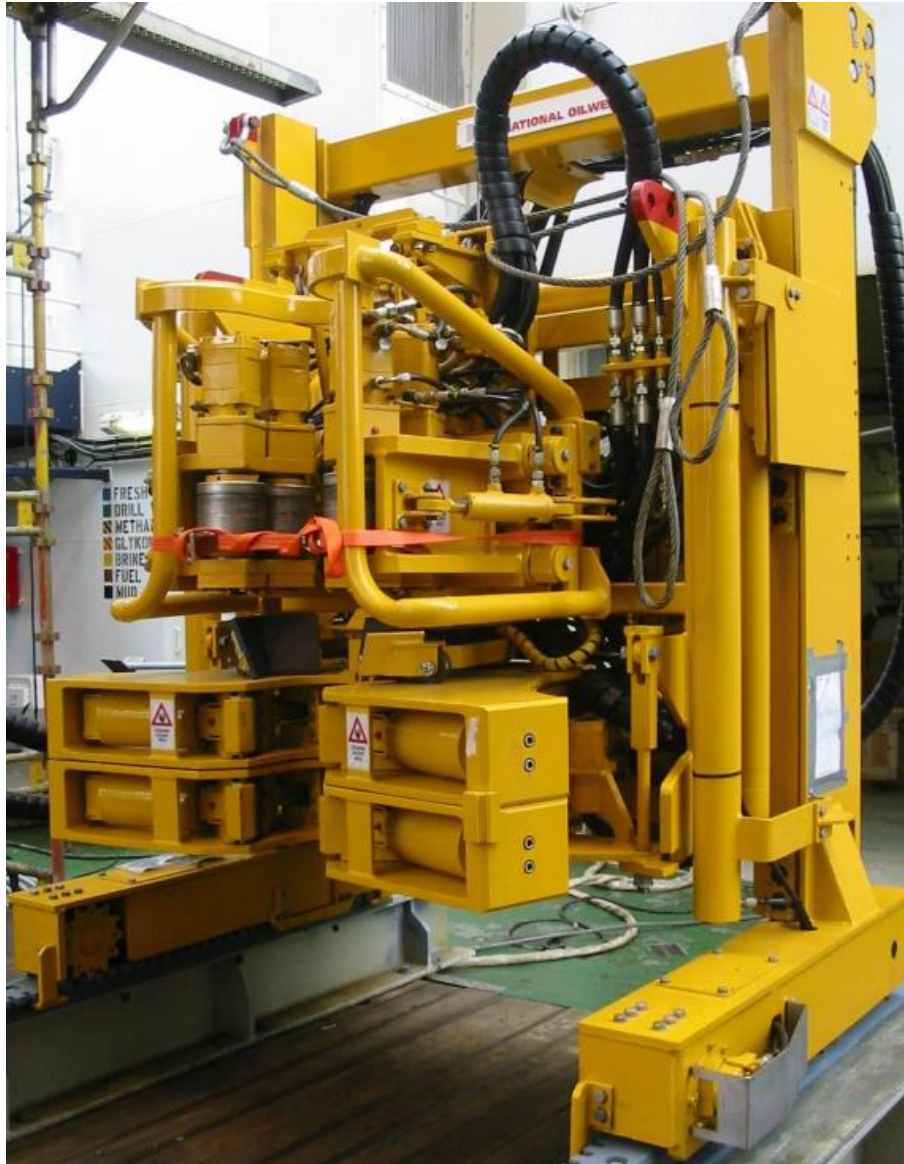
Figure 5-27: Iron rough neck installed on an Island Offshore vessel. [64]
