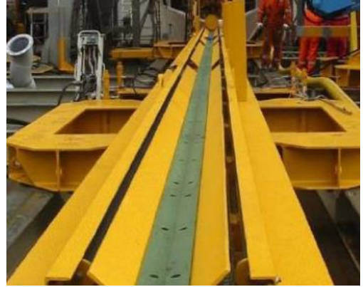
Figure 5-6: Pipe trolley on Island Frontier. [31]
