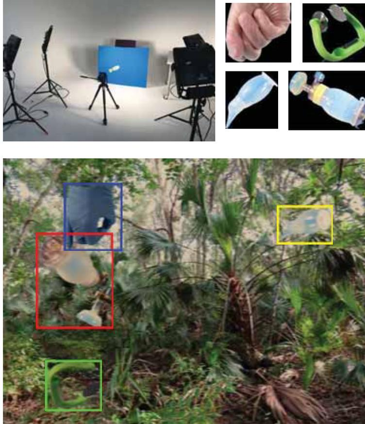
**Figure 4.7:** Illustration of the generation of synthetic images used in object detection training. Top left: Scene for video recording the different objects, top right: Extracted object template examples from the recordings and bottom: a generated synthetic image example.
