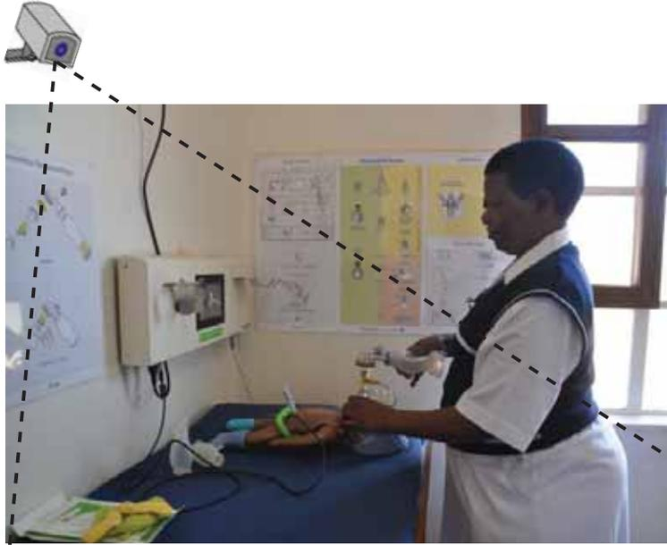
**Figure 4.1:** A newborn resuscitation station at Haydom Hospital in Tanzania [78]. The Laerdal Newborn Resuscitation Monitor (LNRM) is mounted on the wall and attached is the devices Bag-Mask Resuscitator (BMR) and a Heart Rate Sensor (HRS). The camera is mounted on the wall above the resuscitation table. Image reproduced with permission from Safer Births ([www.saferbirths.com](http://www.saferbirths.com)) and modified by the author.
