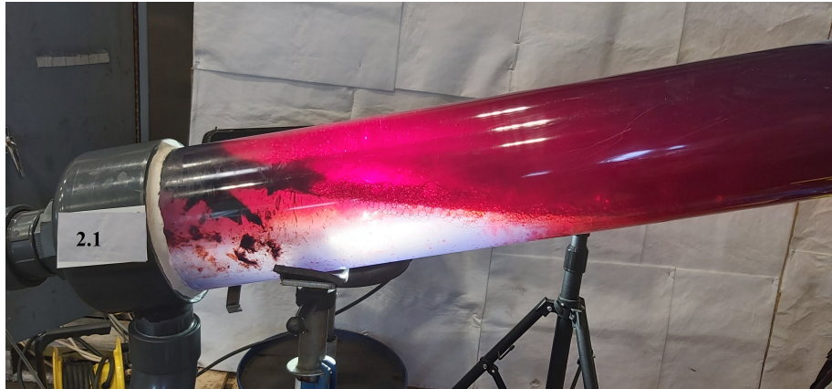
Figure 4.9: Test 2.1- OW flow in an IPIP separator
