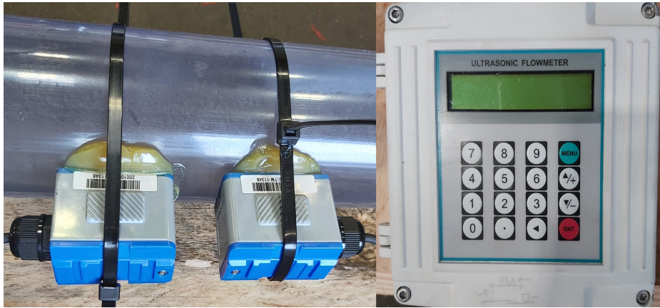
Figure 3.7: Transit-time ultrasonic flow meter and clamp on type transducer
