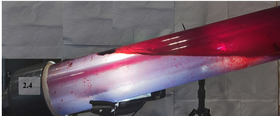
Figure 4.12: Test 2.4- OW flow in an IPIP separator
