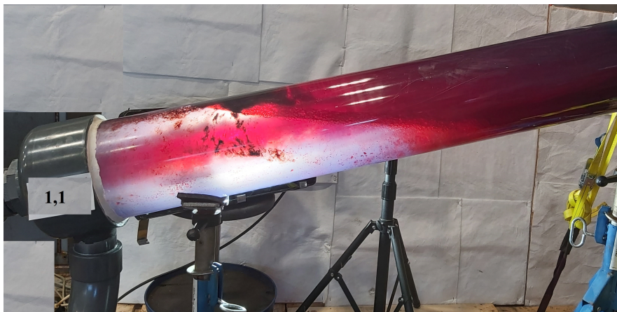
Figure 4.6: Test 1.1- OW flow in an IPIP separator
