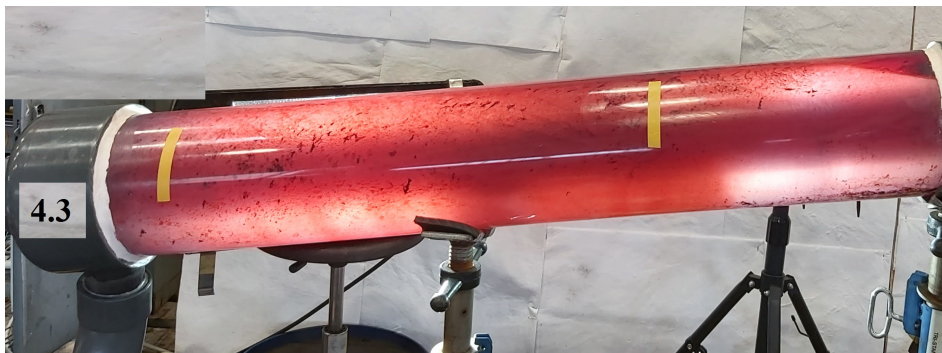
Figure 4.21: Test 4.3- OW flow in an IPIP separator
