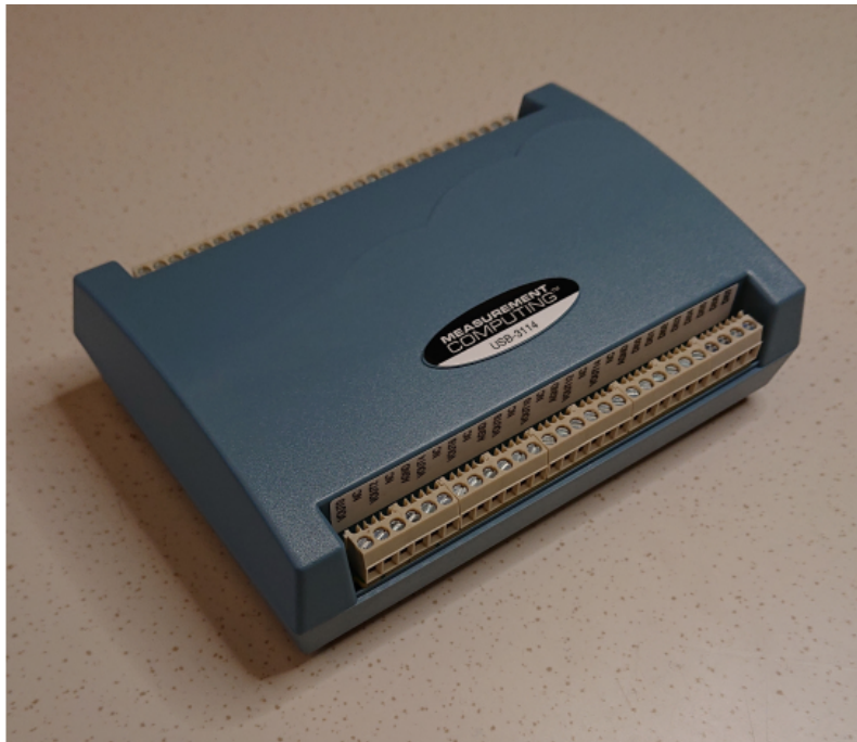
Figure 2.24: Output PLC for the system, USB-3114.
