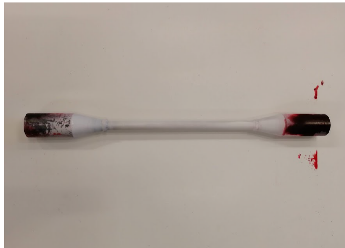
Figure 5.8: Stainless Steel 316 A269 after 138000 cycles in the MTS system, fatigue test.
