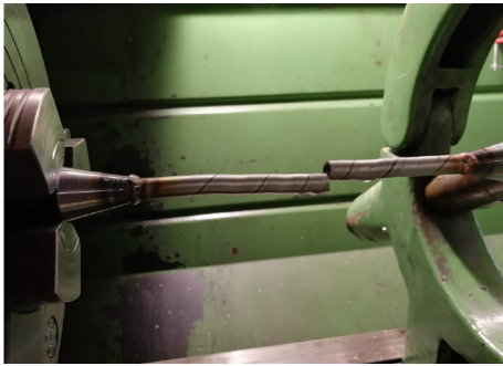
Figure 5.6: Stainless Steel 316 A269 Torsional test.
