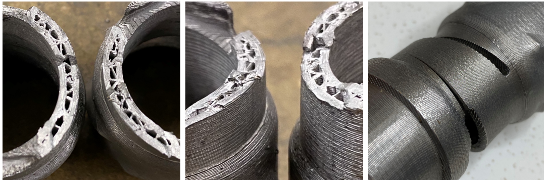
Figure 8.1: Parted bend. One can also see that the bent sub is not solid.
