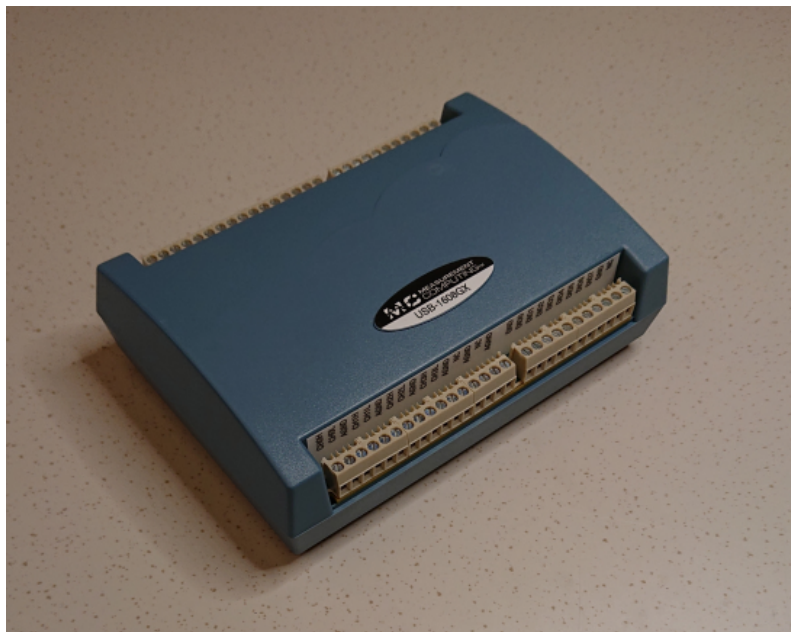
Figure 2.23: Input PLC for the system, USB-1608GX.
