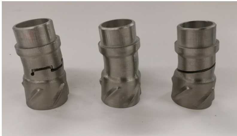
Figure 2.15: 3D printed stainless steel bent subs with different geometries. From left to right; "Lego" cut, no cutout and helical cut.
