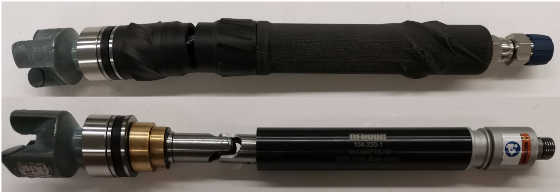
Figure 2.6: Full assembly with and without the exterior.
