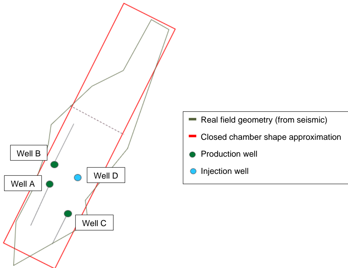
Figure 12. Sketch of the field and approximated shape (rectangle) of closed system.
