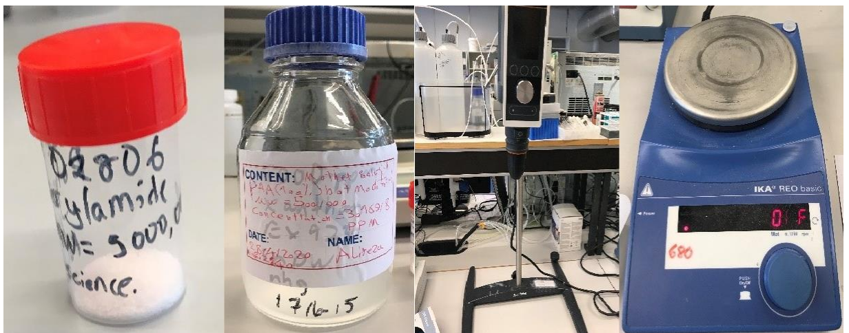
Figure 3.2 from left; HPAM polymer powder ,mother solution C_c=3.10^4 ppm, mixer for mixing polymer powder and water and magnetic mixer
