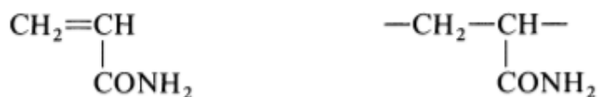
Figure 2.3. Chemical structure of Partially Hydrolyzed Polyacrylamides (HPAM) polymer (Bird, Curtiss et al. 1987)
