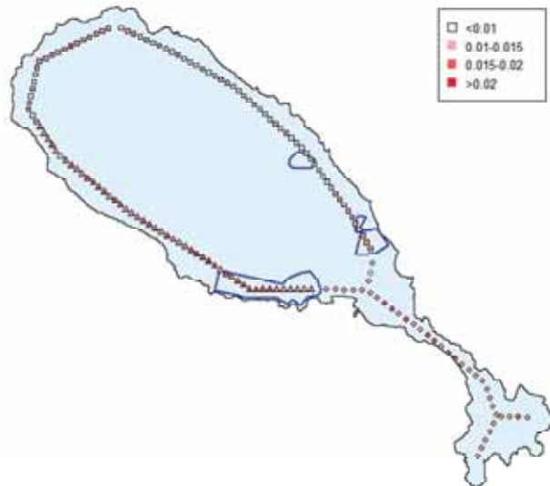
Figure 16: Comparison of the simulated frequency of power node breaks to the areas of St. Kitts that were reported to lose power due to Hurricane Maria.
