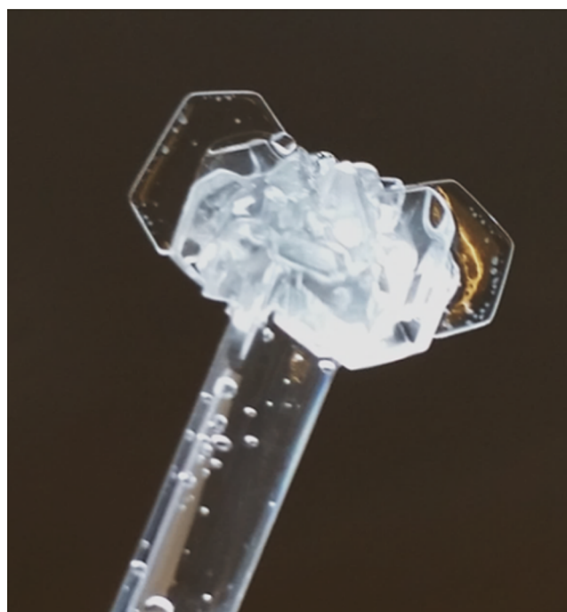
Figure 8. Hexagonal THF hydrate plates from a test with 4000 ppm of polyvinylaminal/ n -hexanal at pH 3.
