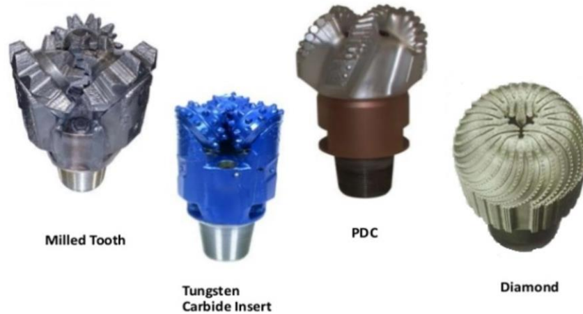
Figure 2.2: Different types of drilling bits; Roller cones to the left and fixed cutters to the right [9]
