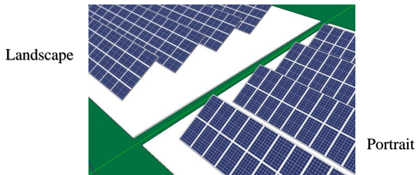
Figure 19: Two orientation alternatives (landscape vs portrait) of solar modules on a rack (simulated image with Energy 3D)
