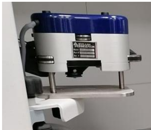
Figure 13 Scanning head of the AFM in unloaded position with the visible short legs.
