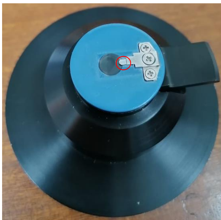
Figure 8 Correctly placed tip (red circle) before placed on the head of the MFP-3D Origin AFM.
