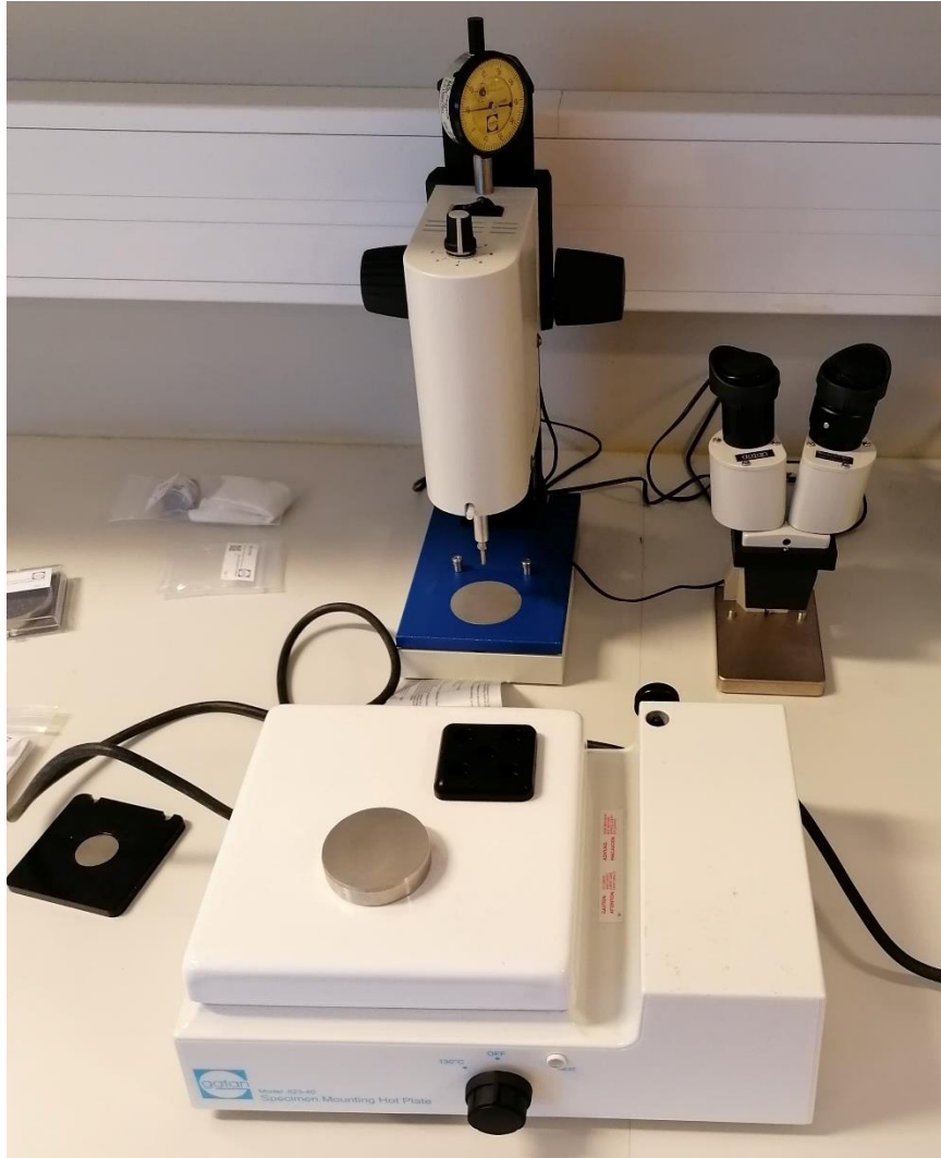
Figure 15 Set-up of the Gatan Model 601 Tuned piezo Cutting Tool. Hot plate in the front (with the specimen table on top), disc cutter back to the left and microscope back to the right.
