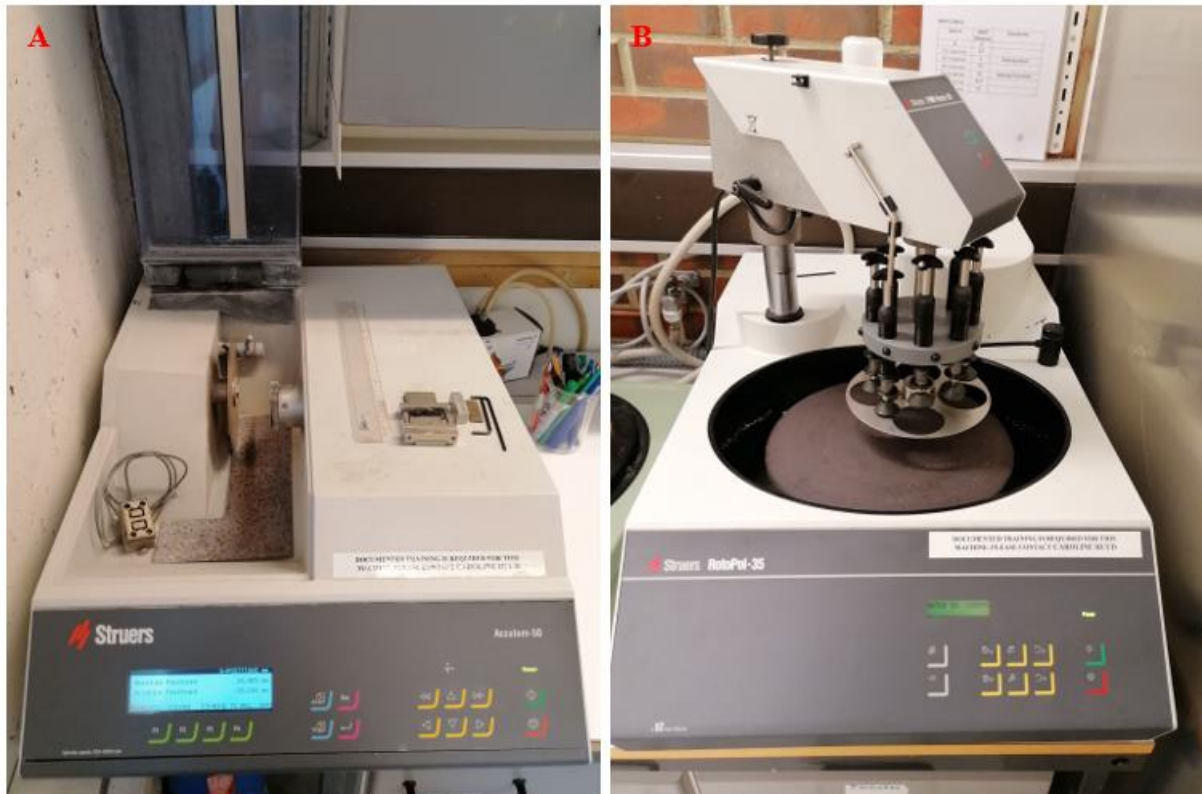
Figure 12 Accutom saw (A) and Struers Rotopol-35 (B) are necessary to cut and polish the samples and mounts.
