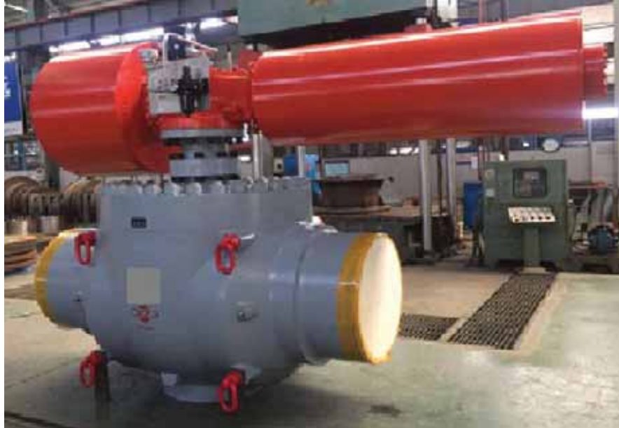
Figure 4: 20" pipeline ball valve for gas export line
