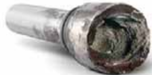
Figure 3: Cavitation attack to a globe valve plug on sealing areas
