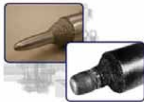
Figure 2: Cavitation Damage in plugs of the globe valves
