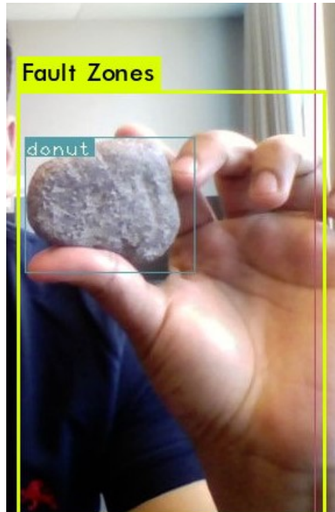
(a) YoloV3 was pre-trained and as a result it detects the irregular caving as a Donut, after training it is correctly detected as "Fault Zones" problem
