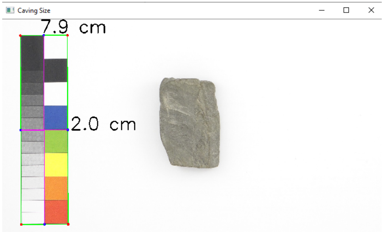
Figure B.2: Measurement of Reference Object
