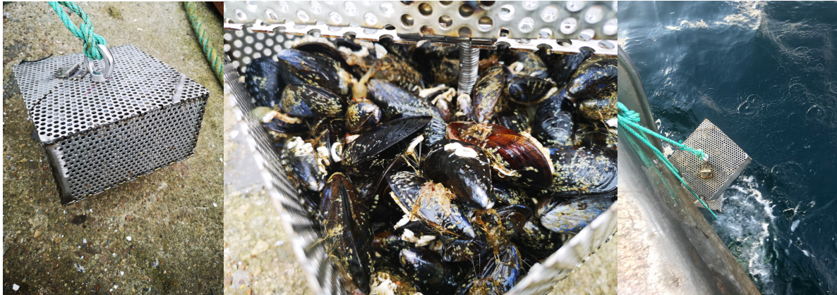
Figure 5: From the left: A picture of the metal cage the mussels were distributed in, the mussels inside the cage, and the caged being deployed at station 1.
