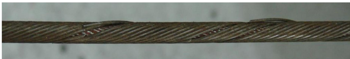
Figure 1.4: Broken Armor wires from H 2 S embrittlement (Moffat et al., 2012)
