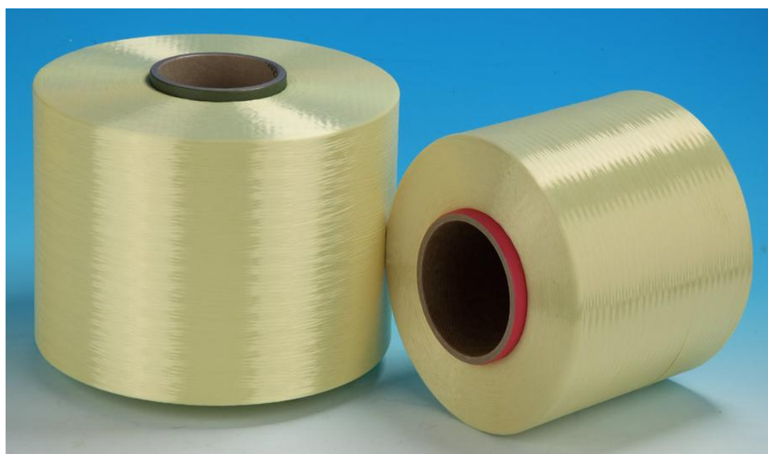
Figure 2.3: Kevlar Yarn in its natural colour (Shanyou Londtai Plastic Products co., ltd)
