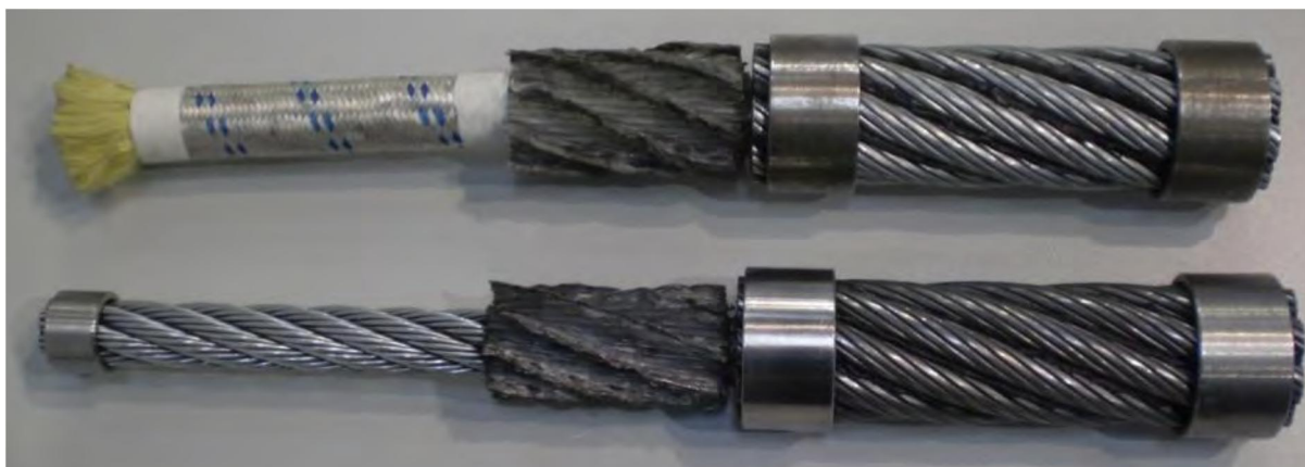
Figure 2.2: Sample composite cable developed by CASAR (Rebel, 2012)
