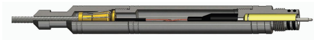
Figure 3.17: Cable Termination in the currently used Monoconductor Cables (Dunning, 2013)
