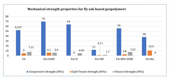
Remarks: FA- Fly Ash; GGBS - Ground Granulated Blast Furnace Slag; K - Kaolin; MK - Metakaolin; BA- Bagasse Ash
