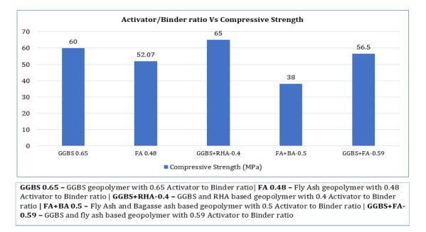
**Figure 5.** Graph showing activator/binder ratio vs compressive strength. Remarks: FA—Fly Ash; GGBS—Ground Granulated Blast Furnace Slag; K—Kaolin; MK—Metakaolin; BA—Bagasse Ash; RM—Red Mud; RHA—Rice Husk Ash.
