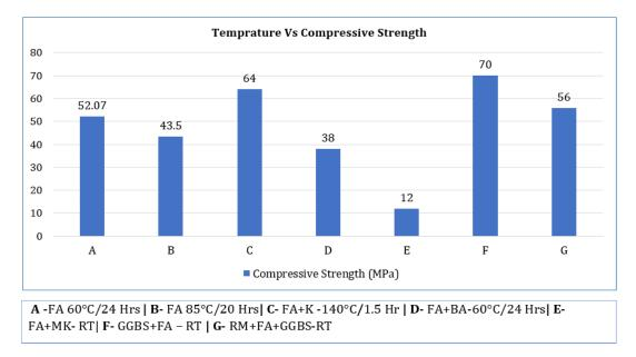
Figure 4. Graph showing temperature vs compressive strength.
