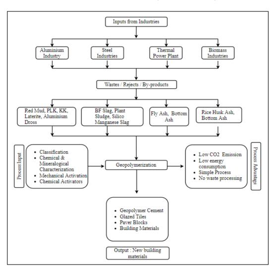
Figure 1. Process diagram for value-addition to industrial wastes through geopolymer synthesis.
