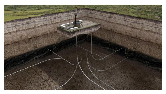
Figure 2.1: Multilateral Wells: Example of a Directional Drilling Application (Butler, 2018).
