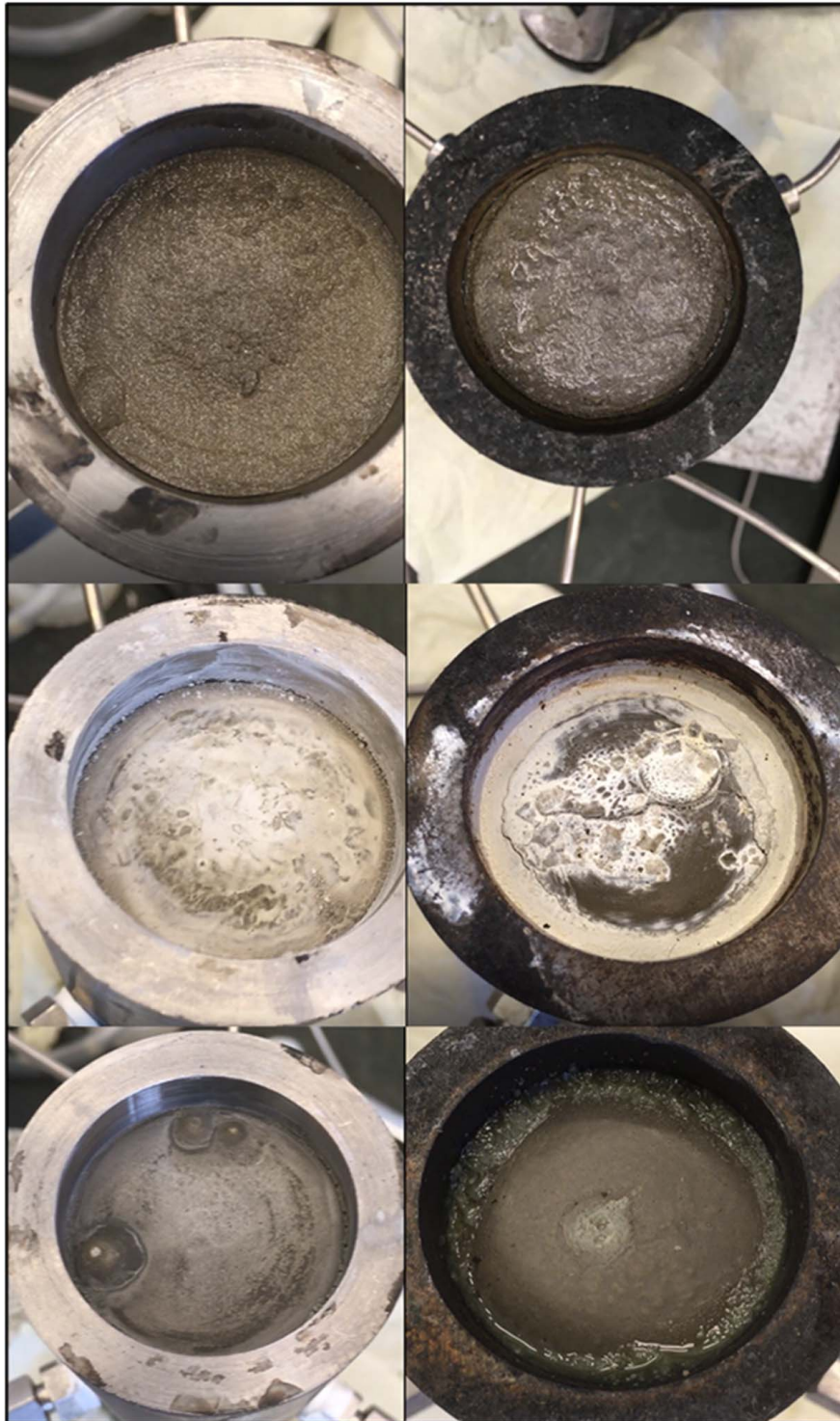
Fig. 10 Top: API neat class G samples started to leak both at interface and within the bulk at 100 psi of differential pressure. Middle: Expansive cement at 500 psi of differential pressure. Bottom: Geopolymer at 500 psi of differential pressure. Both expansive cement and geopolymer revealed no fluid leakage within the bulk.
