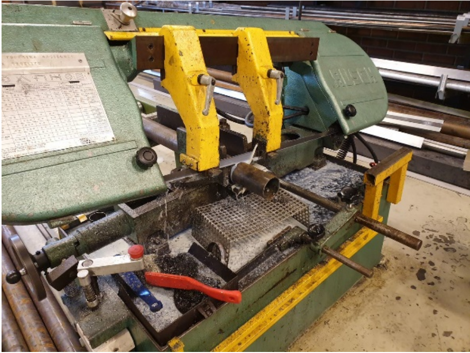
Figure 9: Cutting the pipes
