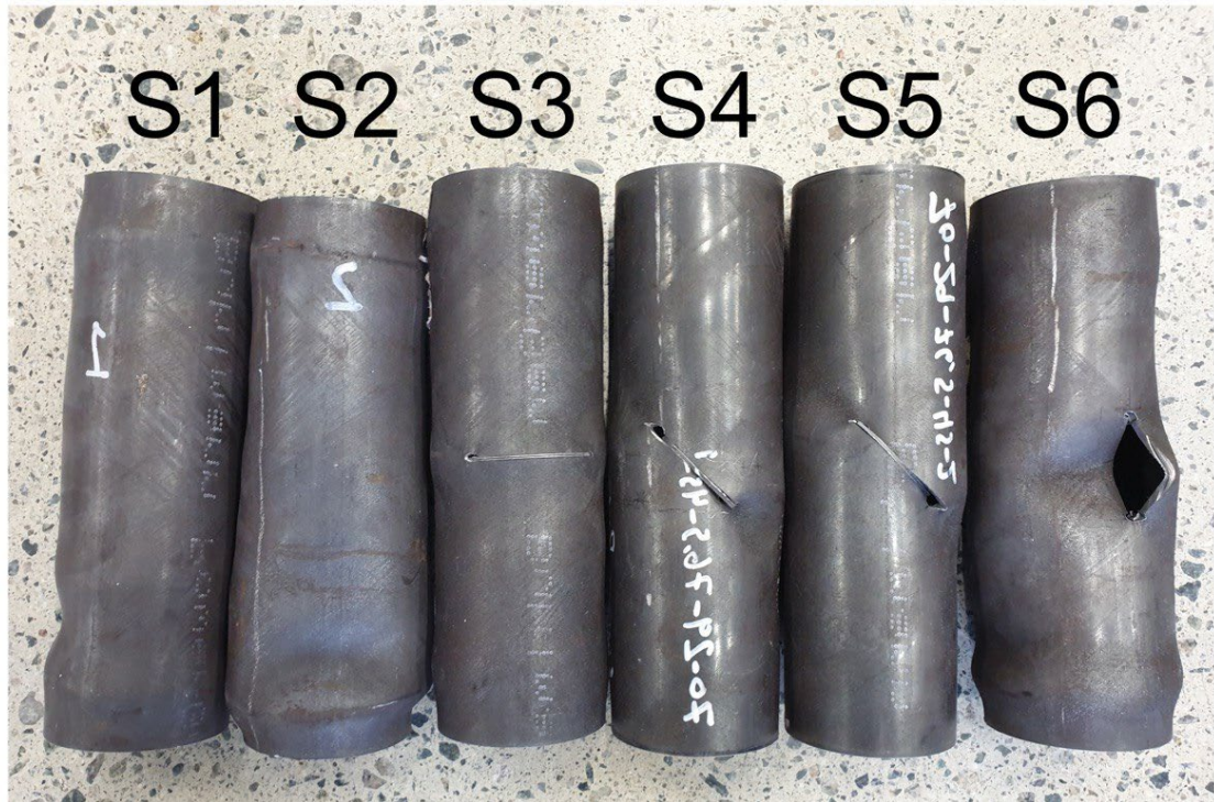
Figure 45: Deformed shape stub columns
