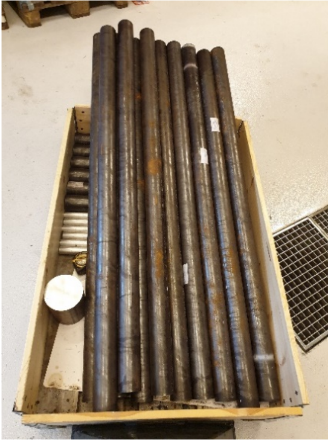
Figure 8: Columns cut from the pipes
