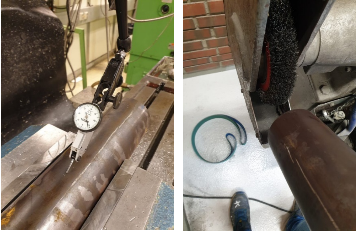
Figure 11: Measuring and brushing of external steel
