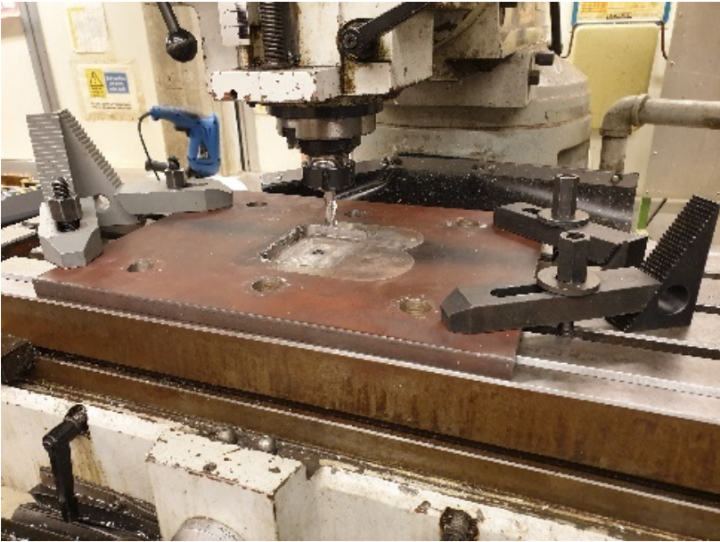
Figure 23: Bottom plate repair
