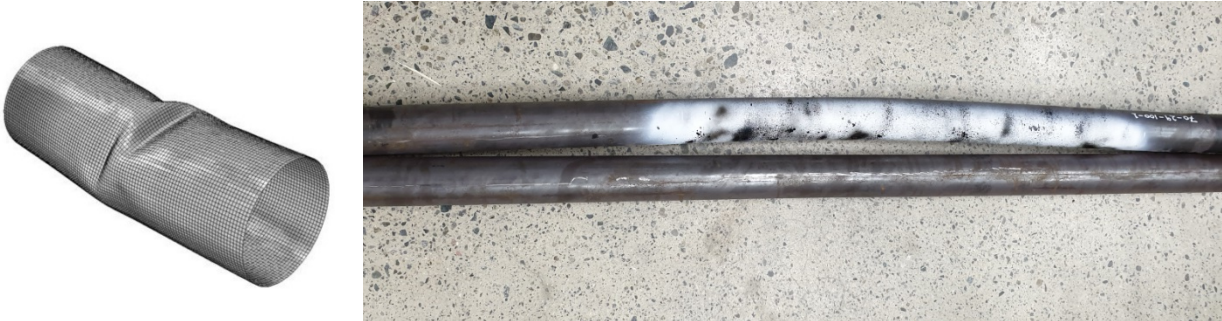
Figure 3: Local and global buckling, respectively (Mic.uth.gr, 2021)
