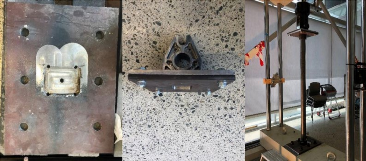
Figure 18: Bottom plate, top plate and test setup used in (Vo T. & Hestholm K., 2019), respectively
