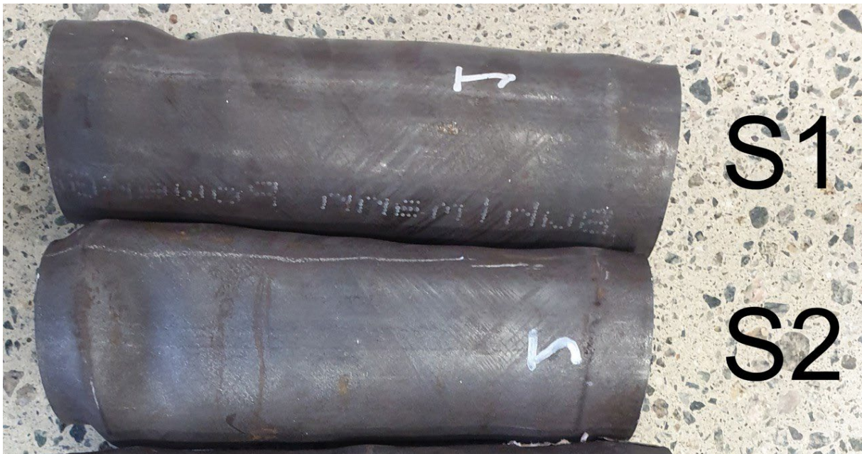
Figure 33: Deformed shape stub columns
