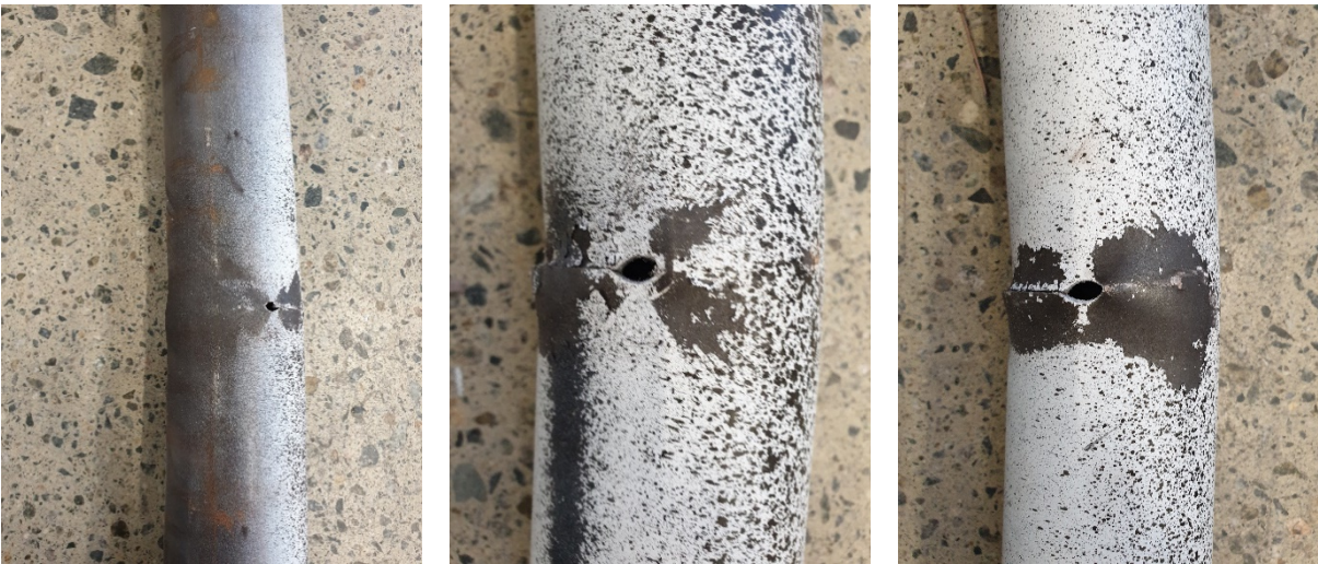
Figure 43: Deformed shape of cracked area (6, 8 and 10mm hole respectively)
