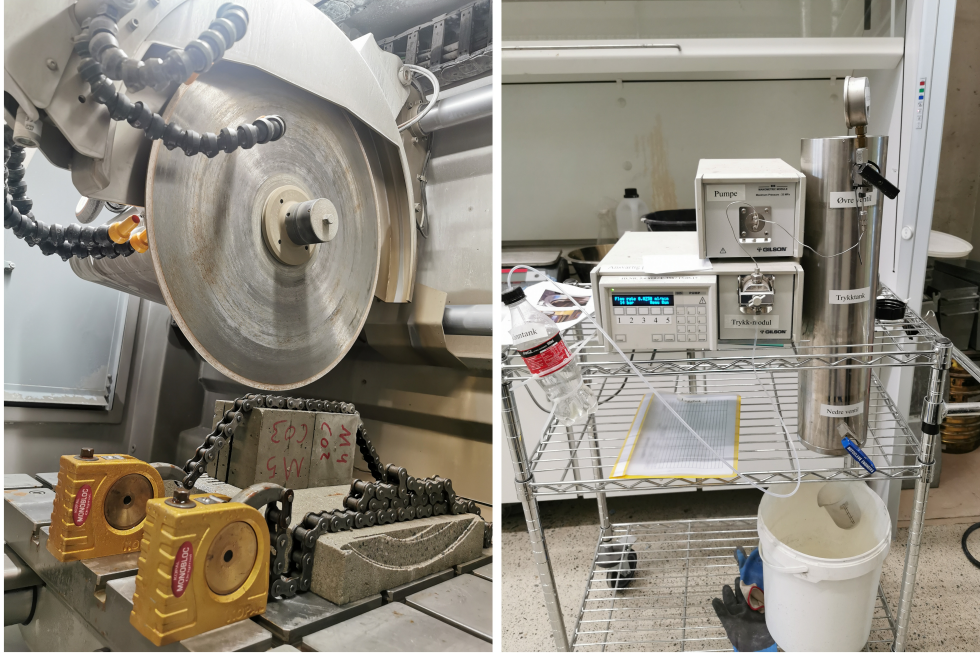
Figure 3.18: Equipment used to carry out the PF-method. The cutting machine is shown on the left and the pressurized tank setup is shown on the right.
