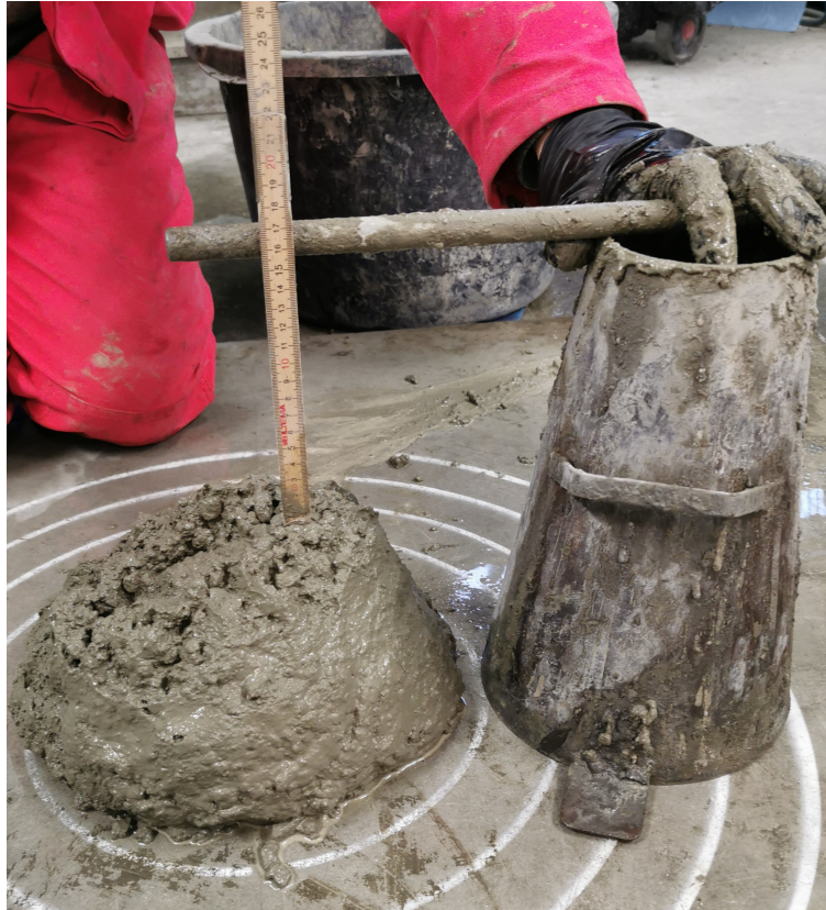
Figure 3.9: Slump test. The slump height is measured after the concrete is allowed to move freely and compared to the height of the cone.
