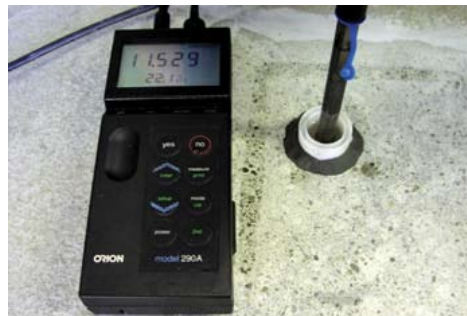
Fig. 9: Measuring pH using a pH probe with a digital meter. Here, the pH is shown to be 11.53
