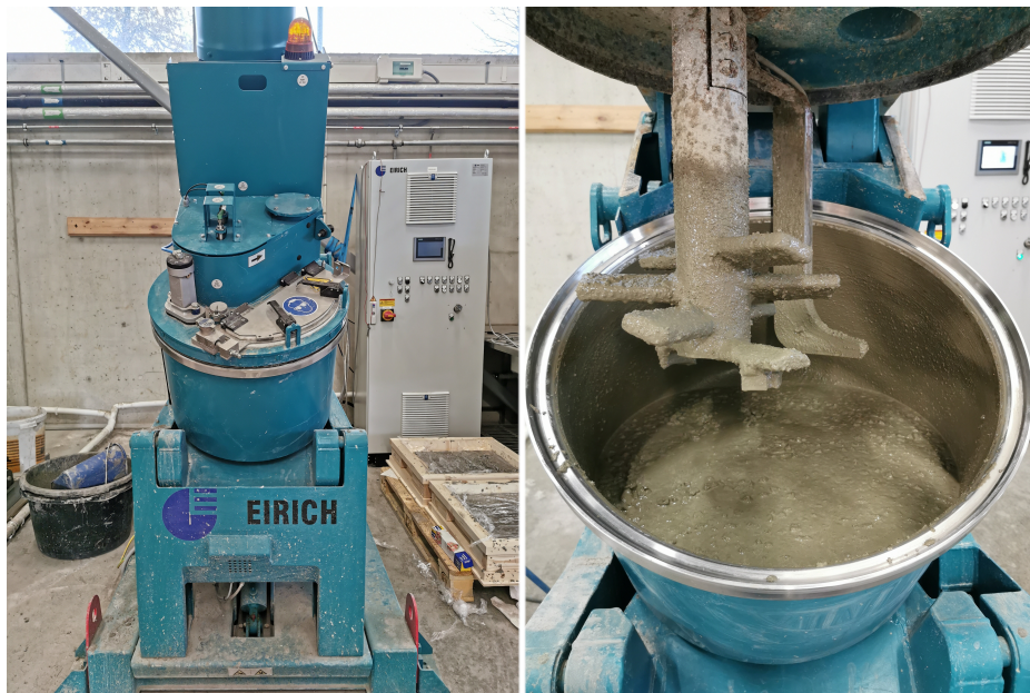
Figure 3.8: Concrete mixer on the left, and the mixing chamber is shown on the right.
