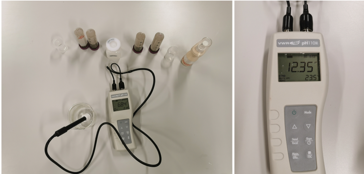
Figure 3.21: Equipment used in pH test to the left and pH Instrument to the right.
