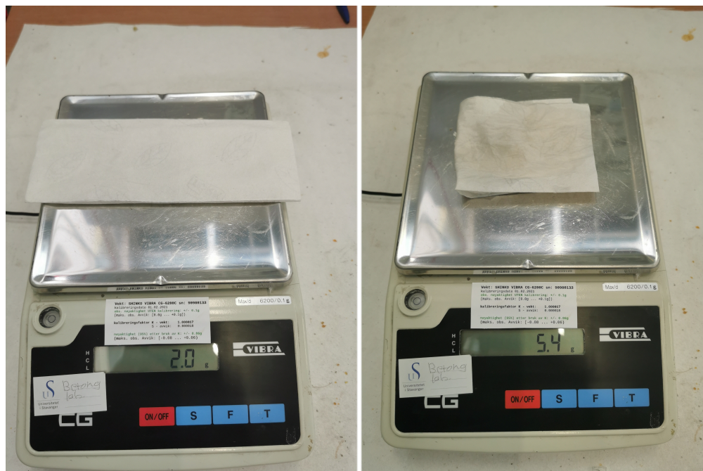
Figure 3.26: Weight gain test "tissue paper". The dry paper (left) is used on the inside of the chamber after carbonation curing and then weighed again (right).
