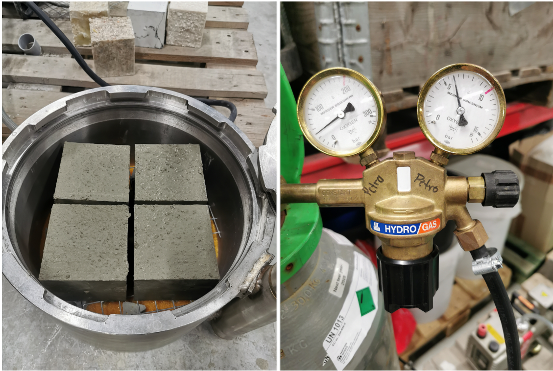
Figure 3.14: Specimens placed inside the airtight chamber to the left and pressure gauges to the right
