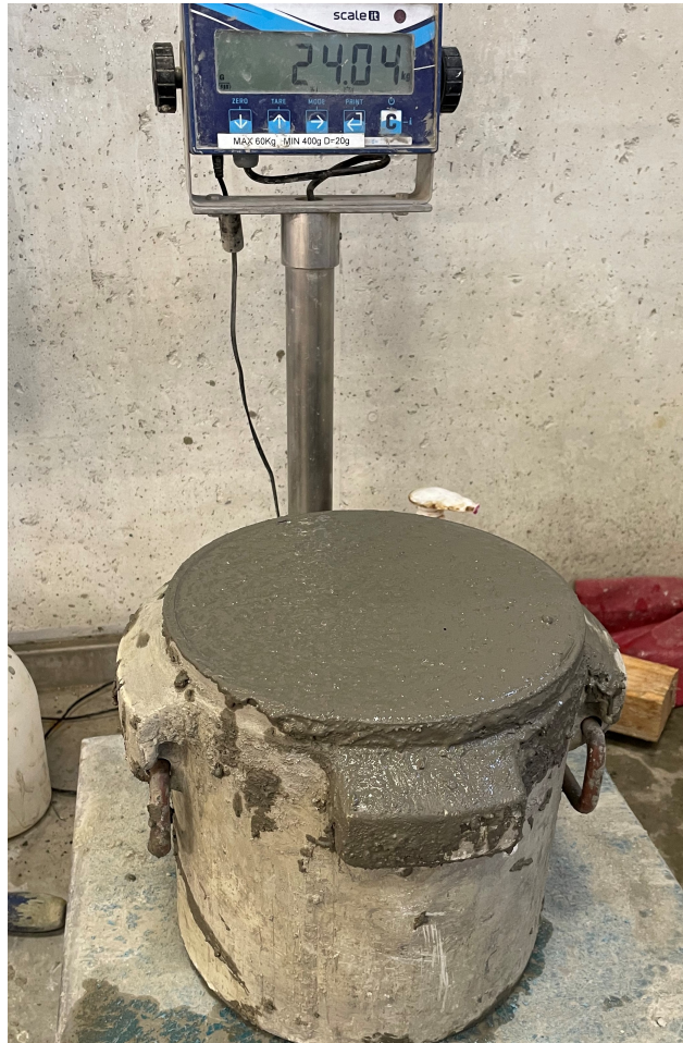
Figure 3.15: Density container filled with fresh concrete
