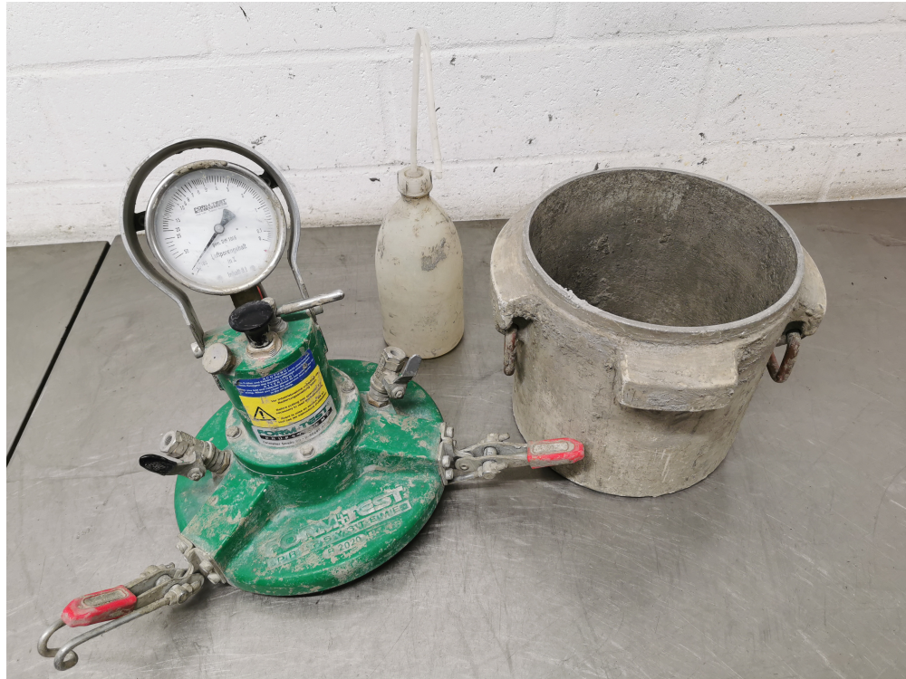
Figure 3.10: Concrete air meter
