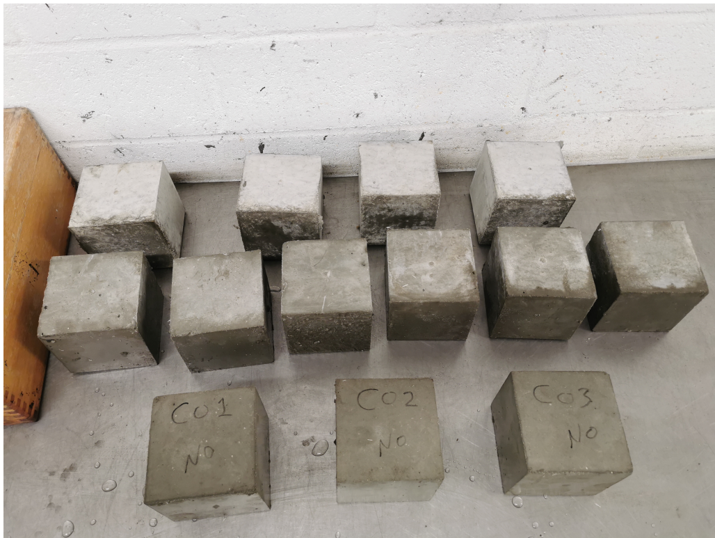
Figure 3.12: Specimens after demoulding
