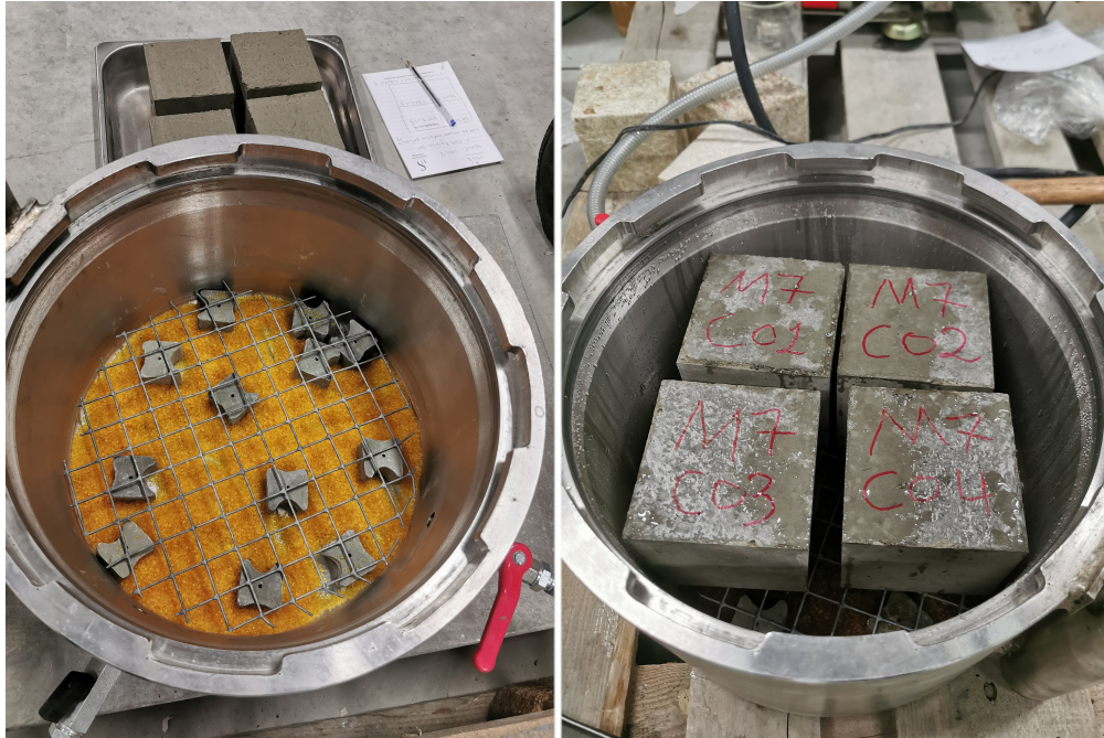
Figure 3.25: Silica gel to the left and water loss to the right. Note the water moisture on the sides of the chamber and on the top of the concrete.
