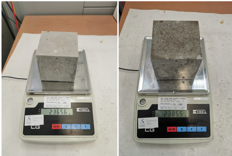
Figure 3.24: Weight gain test "specimen". Measurement before (left) and after (right) carbonation.
