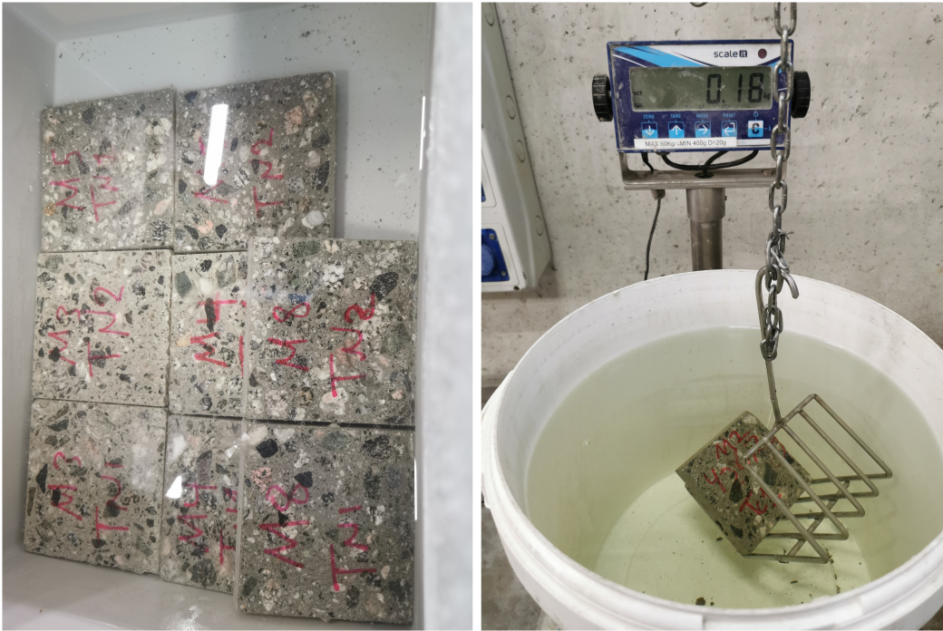
Figure 3.19: Specimen samples placed in water to the left, and typical stirrup arrangement to the right
