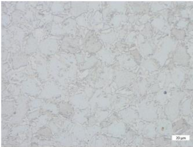
Figure 7. Sample 2. Etched in Kalling 2. Austenite is white.
