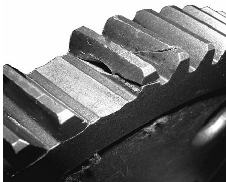
Figure 2.5: Crack initiation due to high load cycles.
