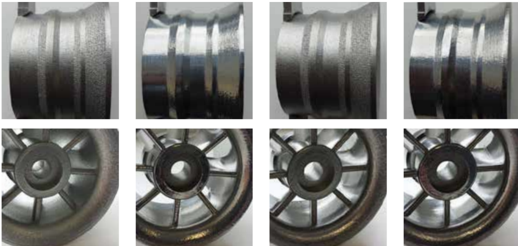
Figure 2.18: Test piece after AFM and COOLPULSE.
