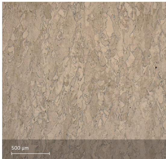
Microstructure solution annealed Etched with etchant Kallings 2
