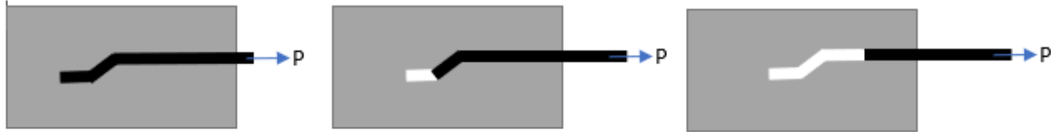
Figure 3-19: How failure by pullout occurs
