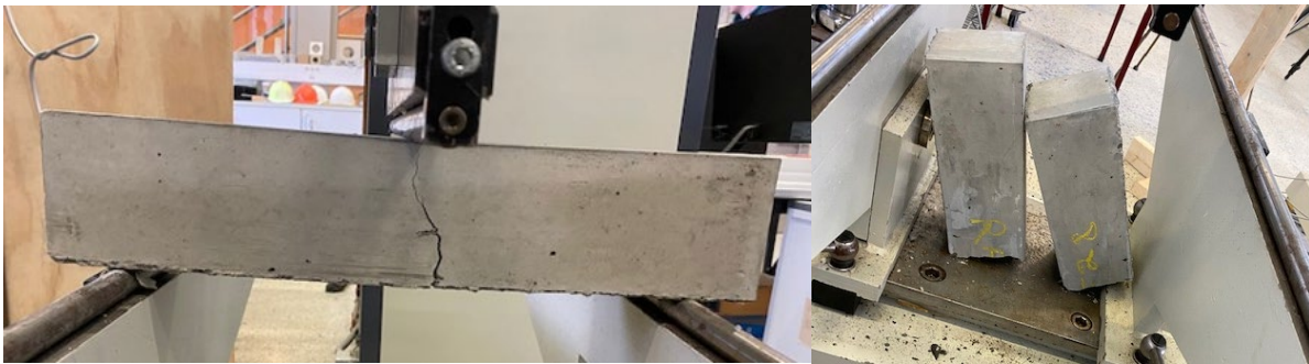
Figure 3-18: Flexural failure of plain concrete a) day 1 specimen b) day 28 specimen
