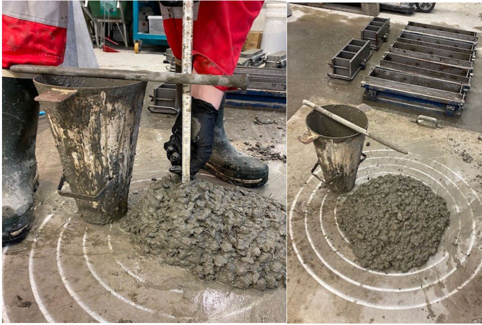
Figure 3-4: Technique used to measure the slump
