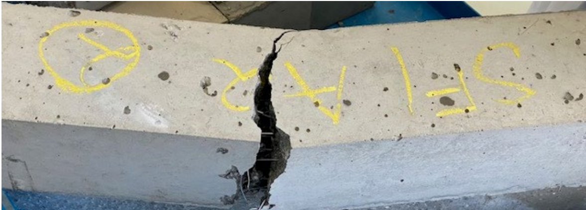
Figure 3-20: Flexural failure of day 28 SFRC specimen
