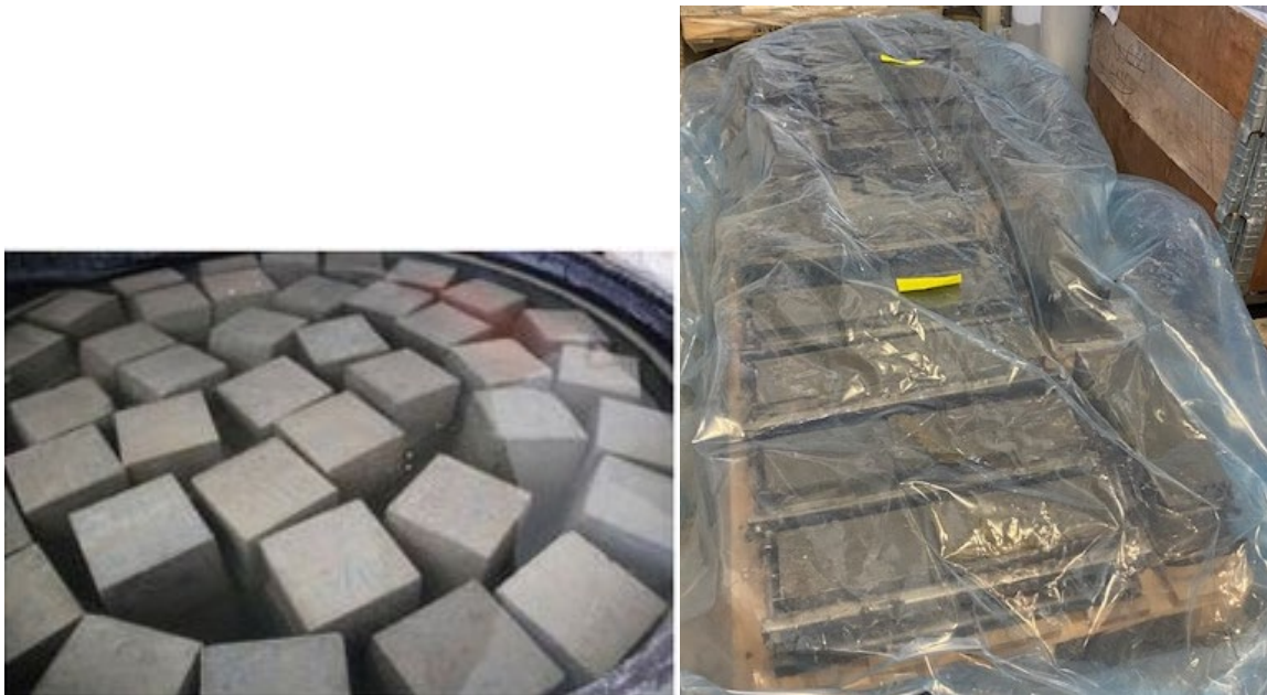
Figure 3-7: Specimens covered with plastic for the first 24 hours of curing and thereafter being placed in a curing tank for the remainder of the curing time.
