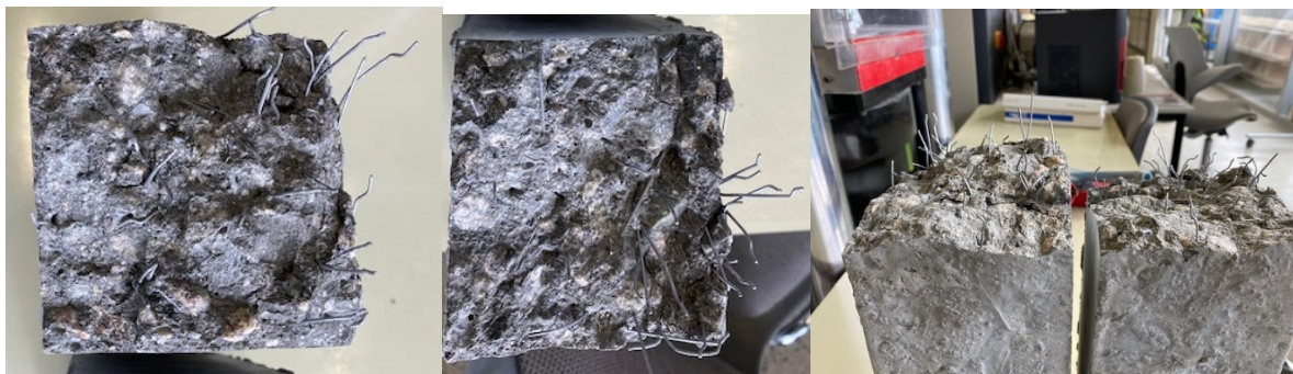
Figure 3-21: Cracked cross section of SFRC specimen
