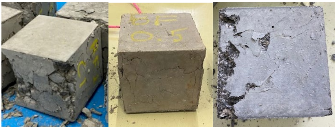
Figure 3-15: Failure mode of a) plain concrete b) BFRC c) SFRC
