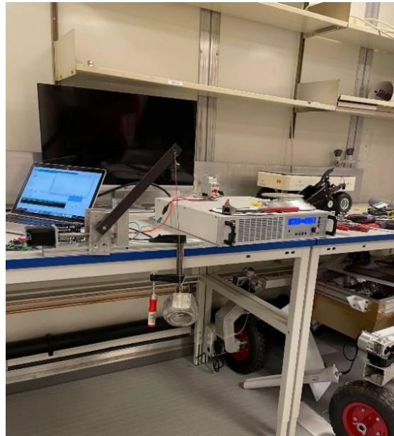
Figure 55 Nema 17 lifting 1774 g at 250 mm
