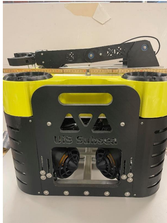
Figure 48 Manipulator on top of ROV
