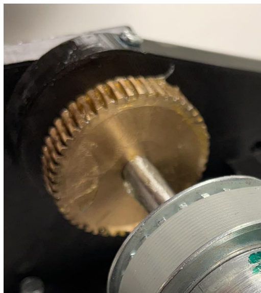
Figure 69 Worm gear press fit
