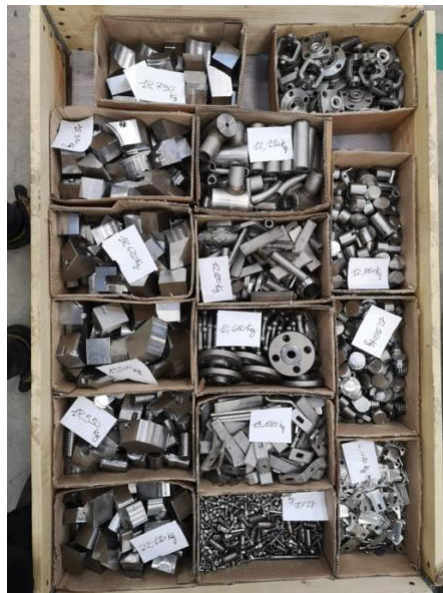
Figure 11: Some of the scrap material used in the atomizing process.
