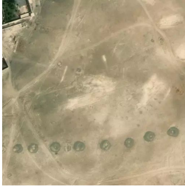
Figure 2.3: Tile from mapbox satellite that shows qanats with the zoom of 17 and the dimensions of 512x512 pixels.
