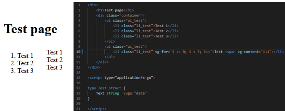
Figure 6.3: Test component as seen in the browser (left) and the code file that generates it (right).
